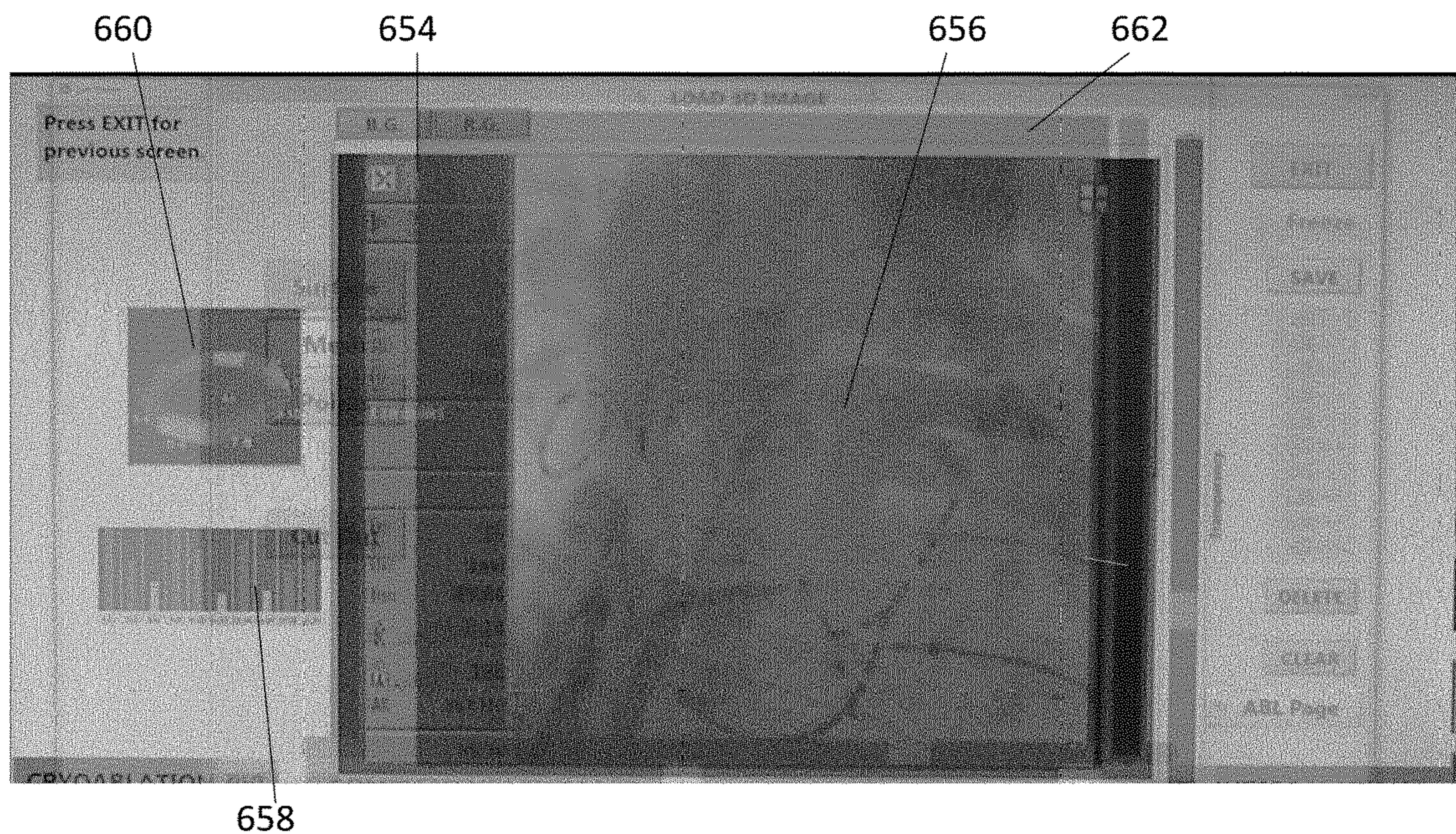
CT overlaid on contrast image with live fluoro overlaid and signals from circ. Catheter (contrast + CT+ live fluoro + signals)
