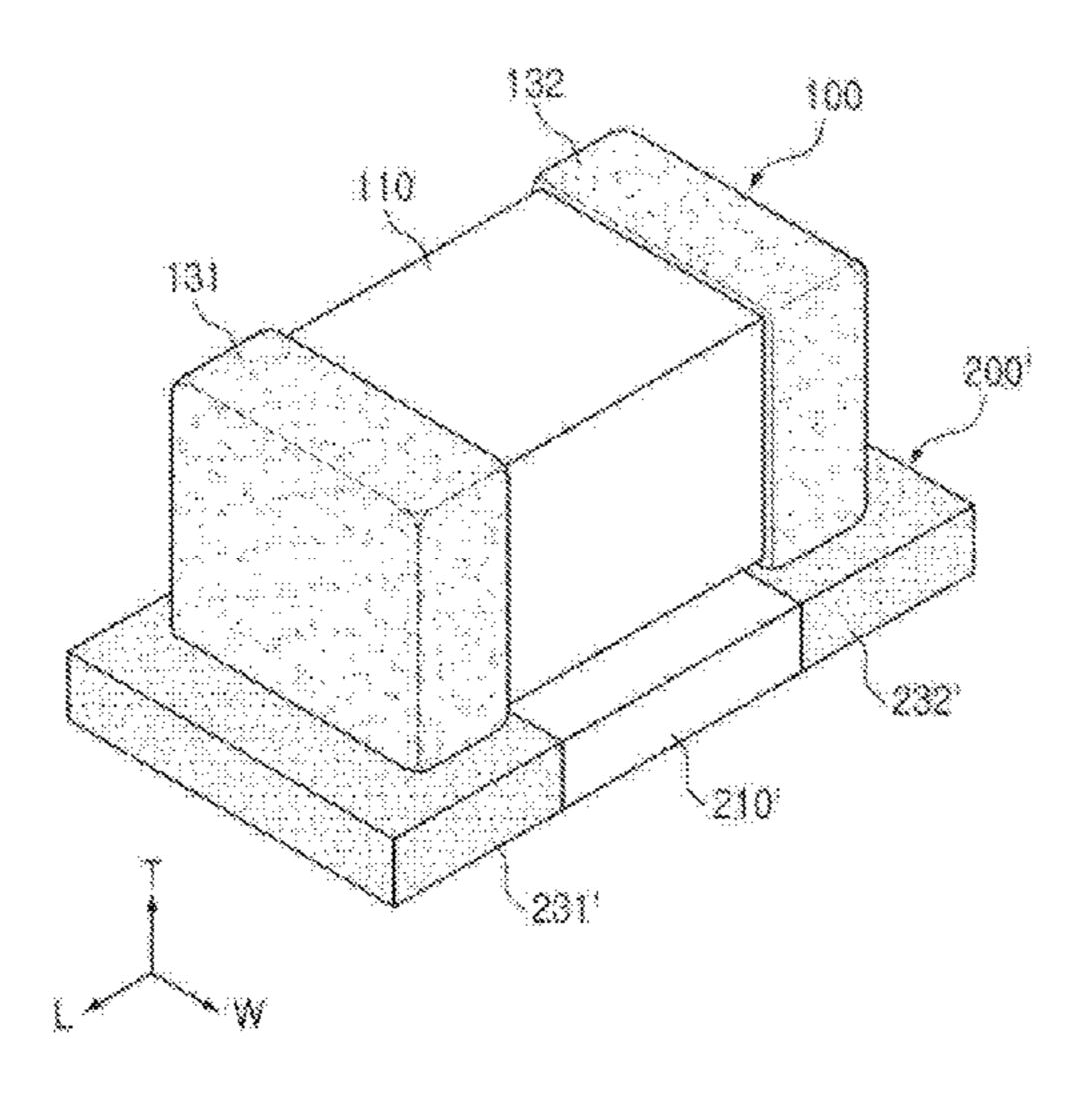
body, and the ceramic chip being disposed on a lower portion of the multilayer ceramic capacitor and formed of a ceramic material having substantially no piezoelectric property, wherein a ratio (T/L) of thickness (T) of the ceramic chip to length (L) of the multilayer ceramic capacitor is selected to minimize vibration of the ceramic chip.
