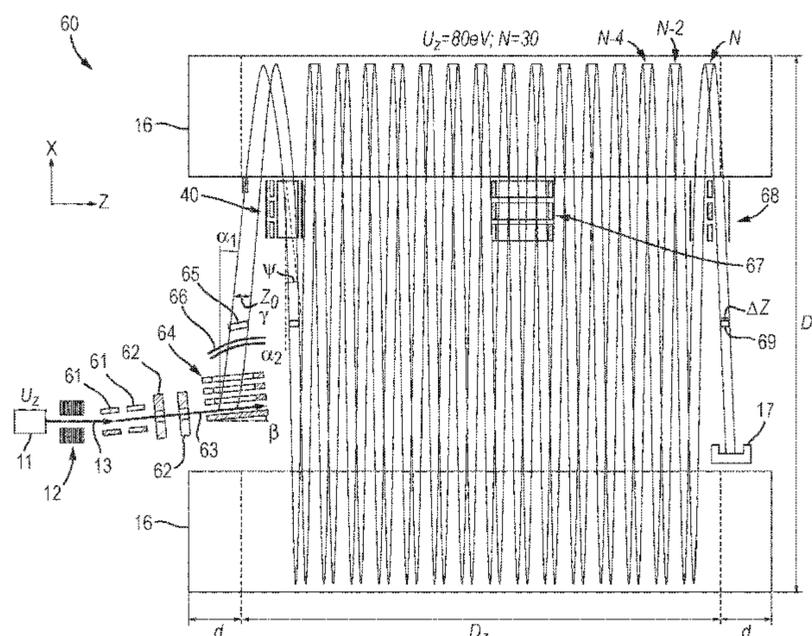
deflector (40) is control by Matsuda plates or other means for producing quadrupolar field in the deflector. Interference with the detector rim is improved with dual deflector (68). The proposed improvements allow substantial extension of flight path and number of ion turns or reflections. The problems of analyzer angular misalignments by tilting of ion mirror (71) is compensated by electrical adjustments of ion beam (63) energy and deflection angles in deflectors (40) and (68).
