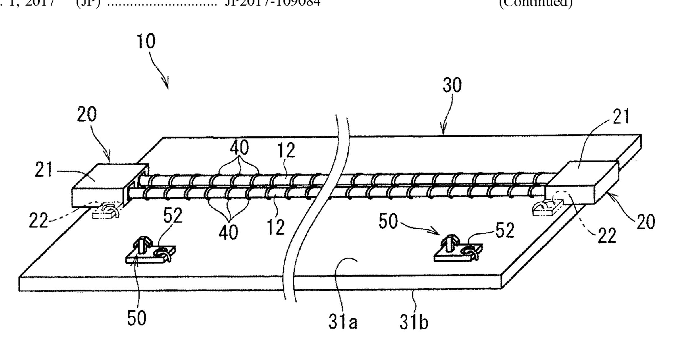
tional exterior component is shaped into a sheet. The electric wire is disposed on one main surface of the functional exterior component. With the thread the electric wire is sewn on the functional exterior component.
