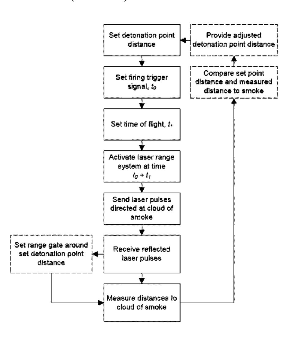
burst of the airburst munition, processing the reflected laser light and defining a range of distances to the cloud of smoke, and setting a range gate around the set detonation point distance prior to processing received reflected laser light within the range gate for limiting the resulting range of distances and cancelling echoes from surrounding terrain.
