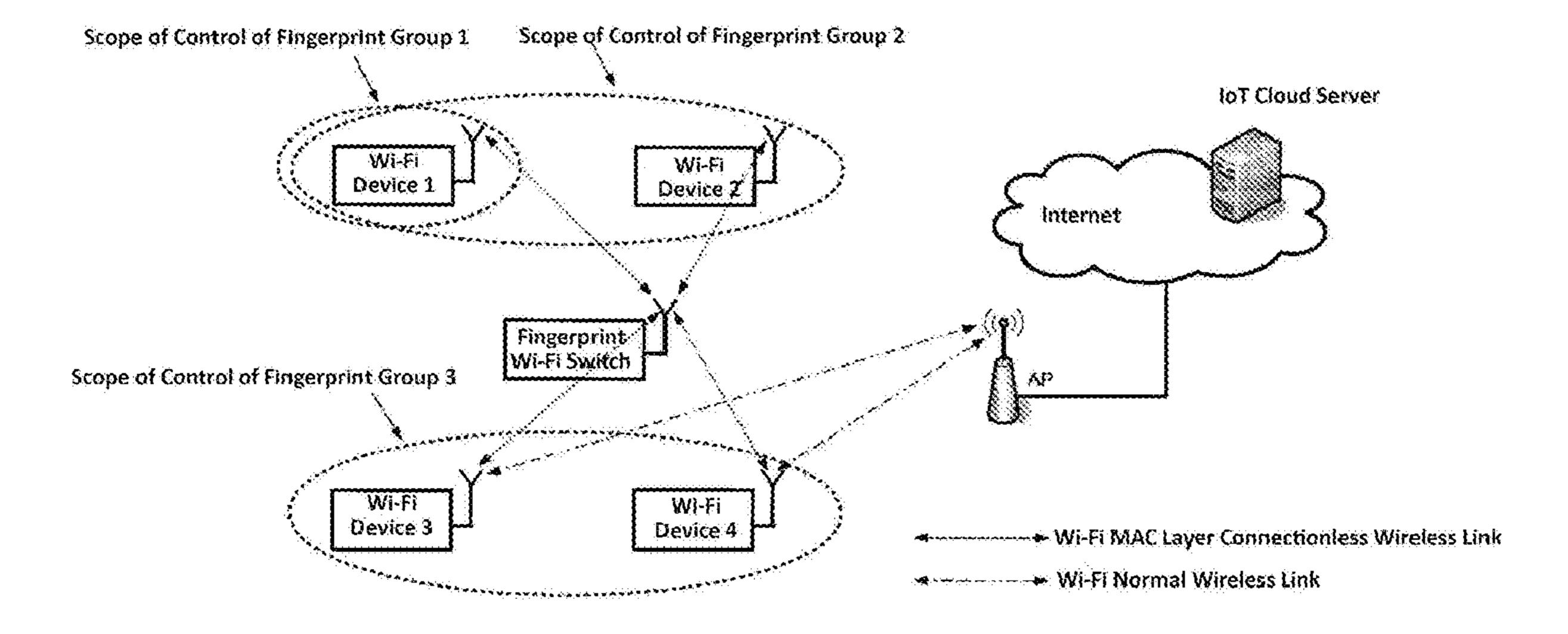
control modes may be freely combined with each other, thereby providing wide applicability. The wire-free finger-print Wi-Fi IoT switch may complete the translation of control information to the standard Wi-Fi IoT device by sending least number of packets, so as to realize low power consumption control. The wire-free fingerprint Wi-Fi IoT switch may also connect to an internet server via a Wi-Fi access point to perform update and upgrade of firmware, fingerprint feature information list, etc.
