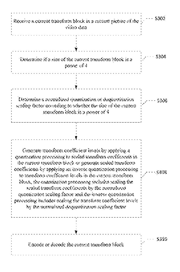
factor and the inverse quantization processing comprises scaling the transform coefficient levels by the normalized dequantization scaling factor.
