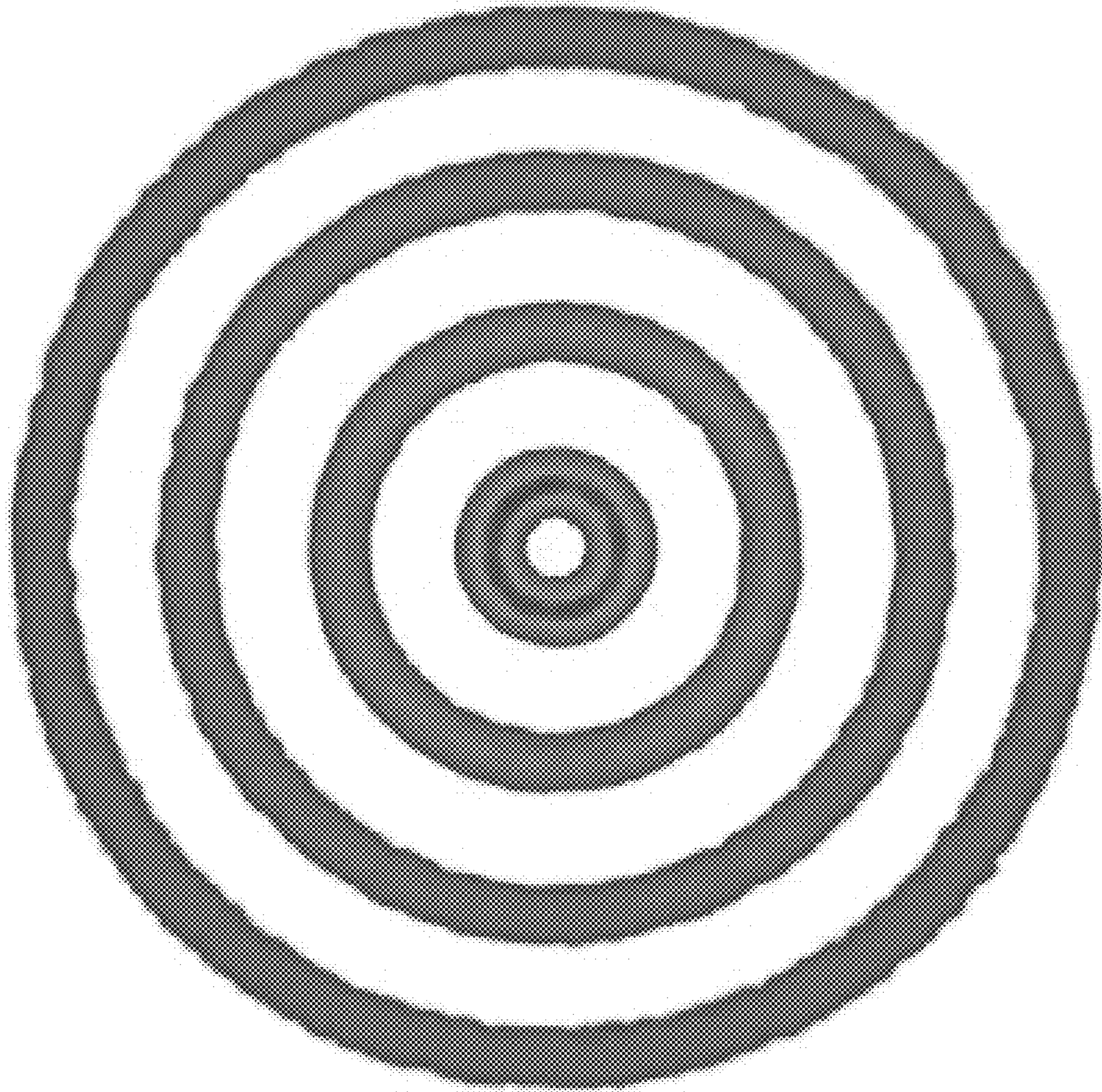
Fig. 8 Optical output profile of SDM
