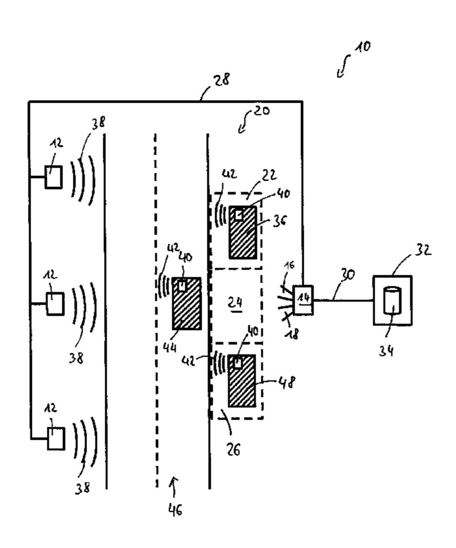
registration server which determines a parking fee on the basis of a tariff for the parking space area which is used and, if necessary, initiates a payment process.
