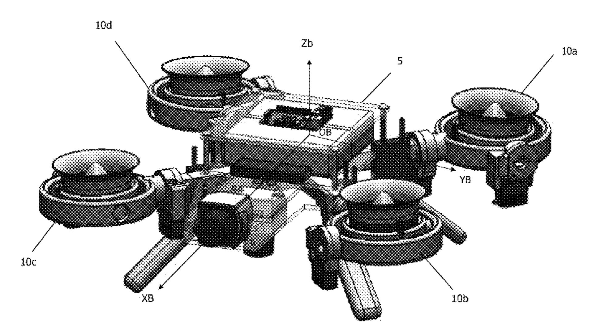
converge the multicopter towards the target characteristic(s), wherein the control algorithm is based on the decoupled mathematical model such that each thruster control variable can be adjusted independently.
