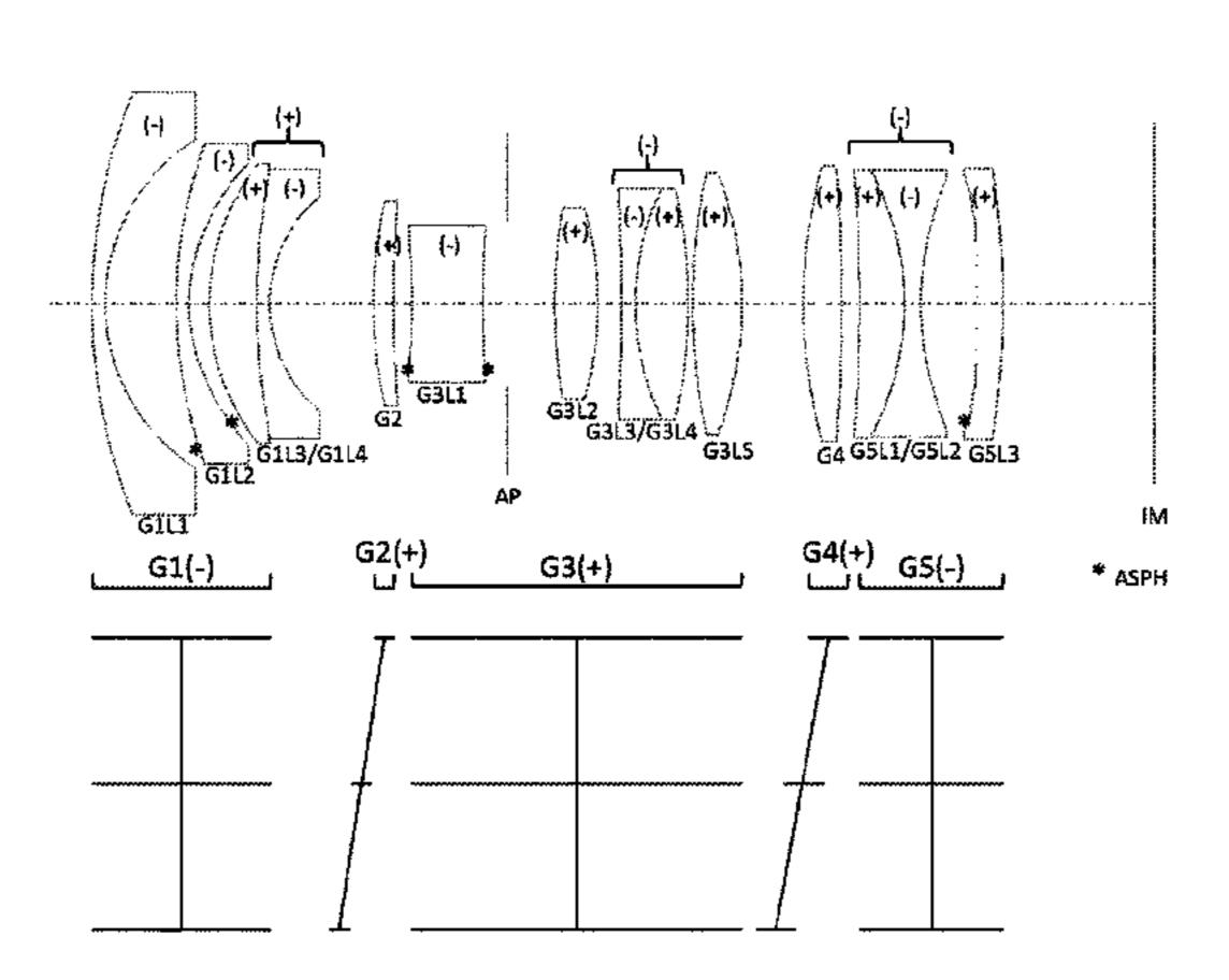
different object distances. The front lens-element group and the back lens-element group have a negative refractive power.
