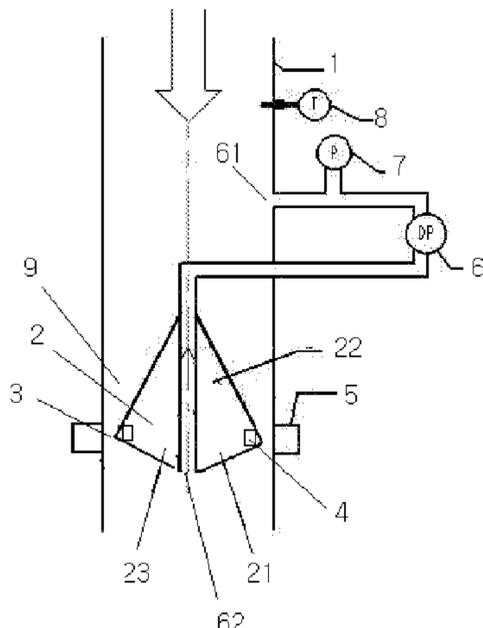
block can transmit radially through the annular gap to reach the gamma ray detector located outside the cylindrical pipe.
