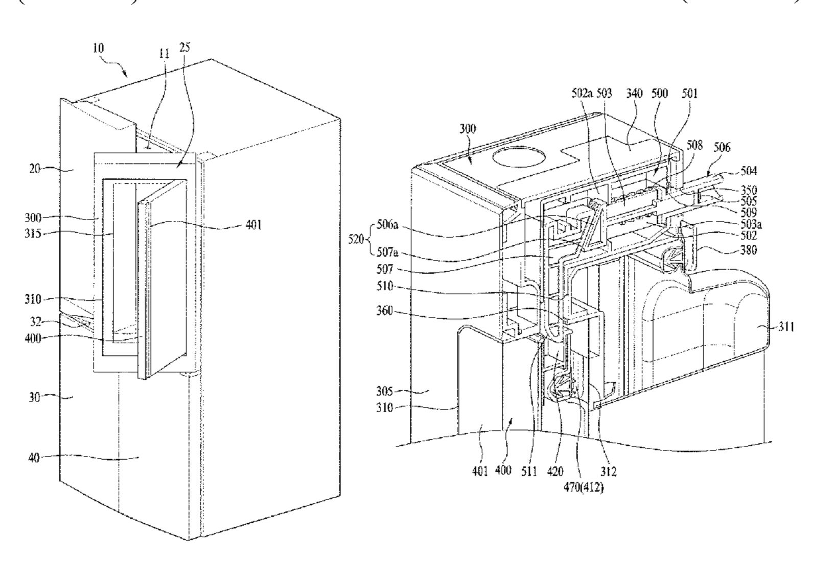
locking device includes a moving member, the displacement of which is changed depending on the open or closed state of the first door, and a catching member, the displacement of which is changed depending on the displacement of the moving member, whereby the protruding length of the catching member from the door frame is changed, the catching member being selectively caught in the catching part.
