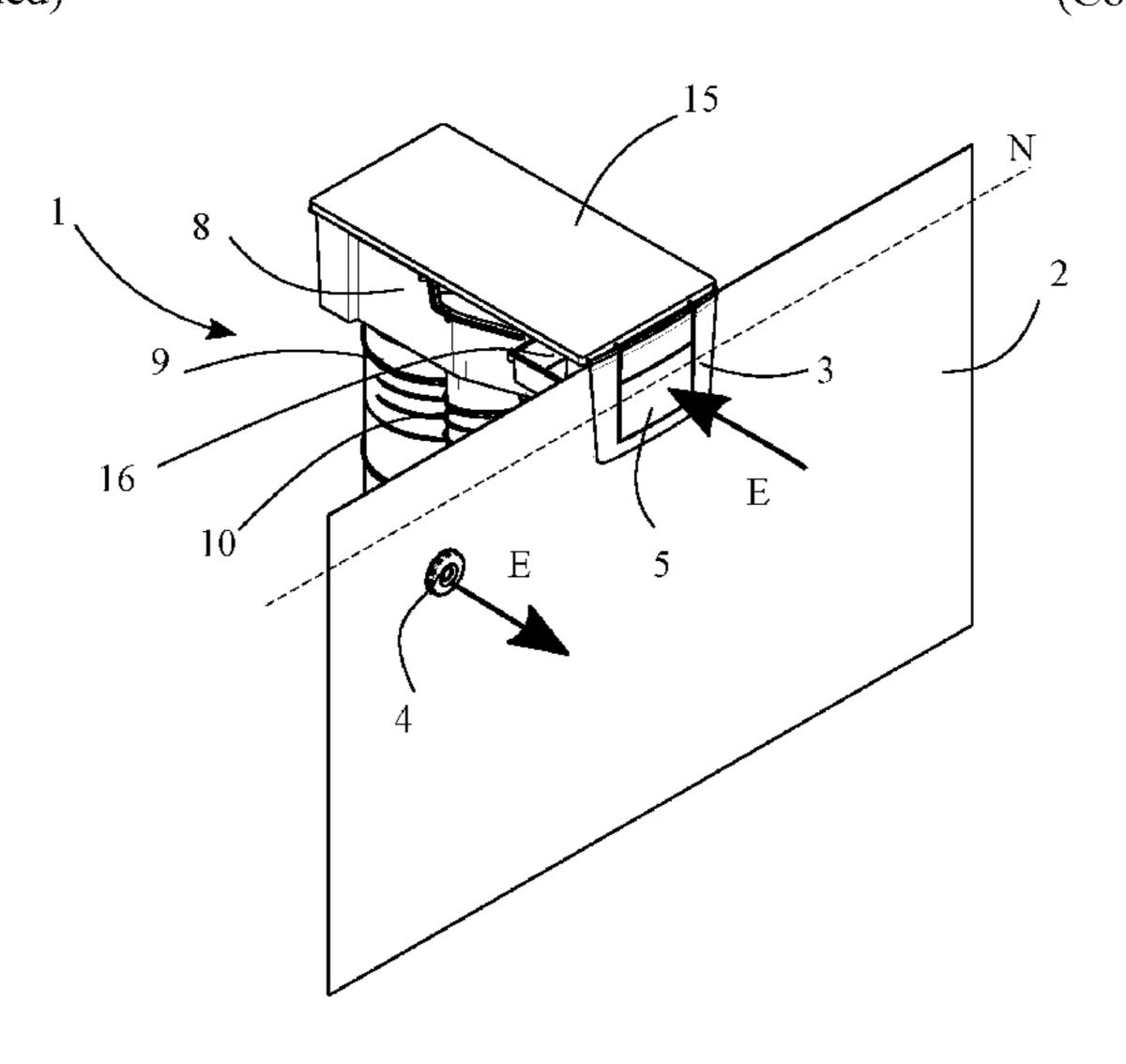
electric motor is a sealed, brushless, autonomously controlled motor that is powered at very low voltage and that may advantageously be immersed inside the filtration unit below the level of the water contained in said pool, thereby enabling said motor to be cooled and sound-proofed naturally by the forced flow of the water from the pool, thereby forming a filtration unit and a pool that have low energy consumption.
