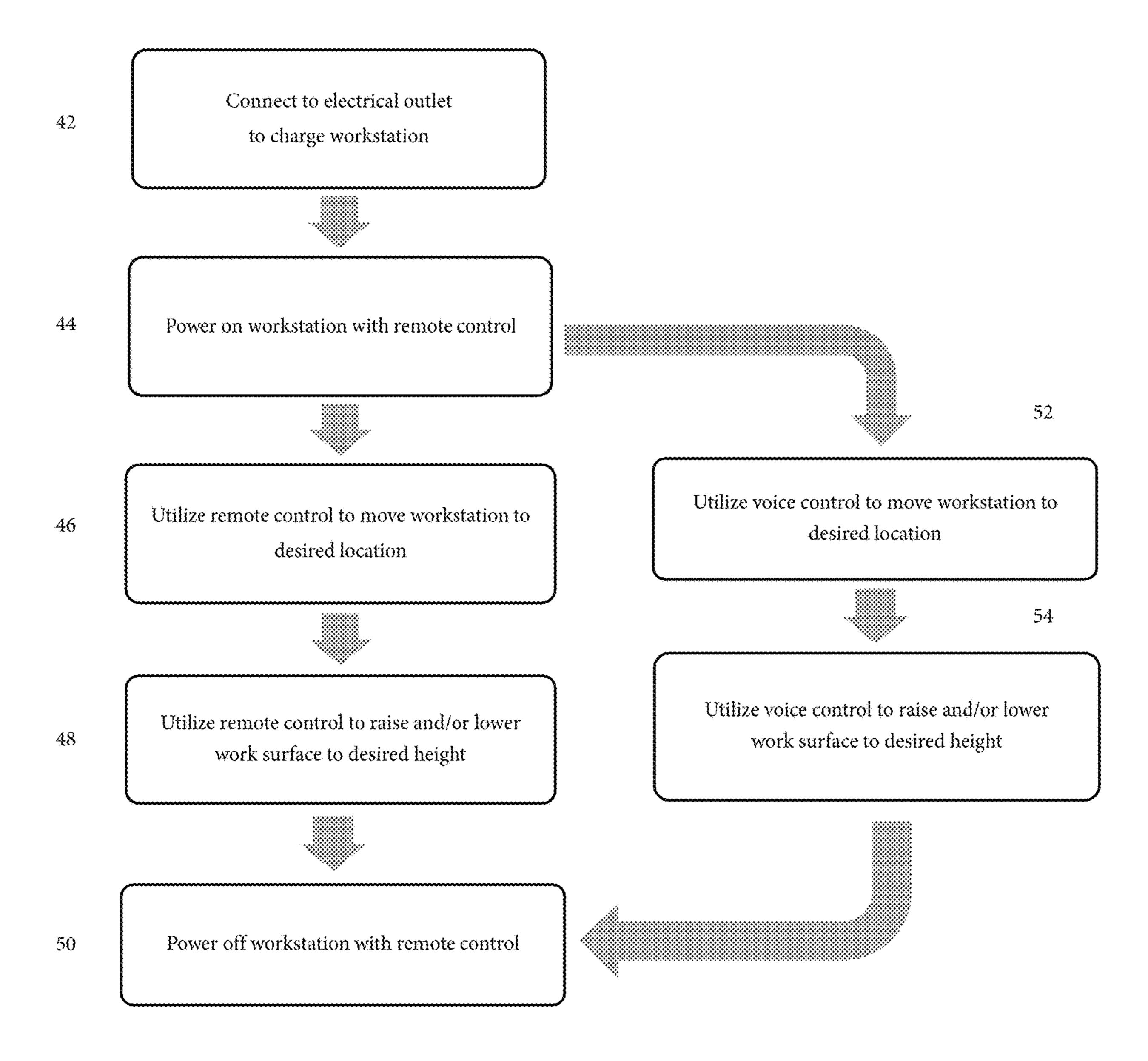
Block diagram of workstation operational concept
