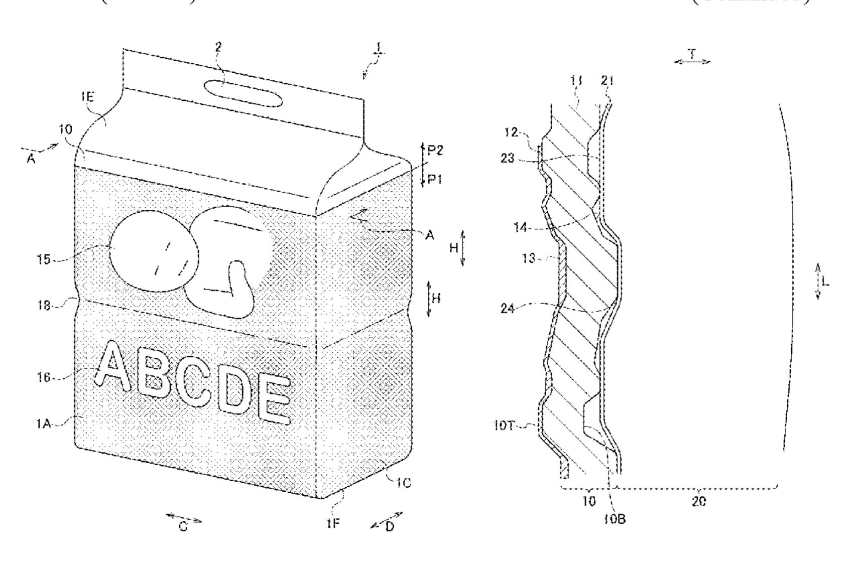
body and comes into contact with the absorbent articles. The surface of the packaging sheet has a plurality of surface recesses formed so as to be recessed toward the back surface side and the back surface of the packaging sheet has a plurality of back surface recesses formed so as to be recessed toward the surface.
