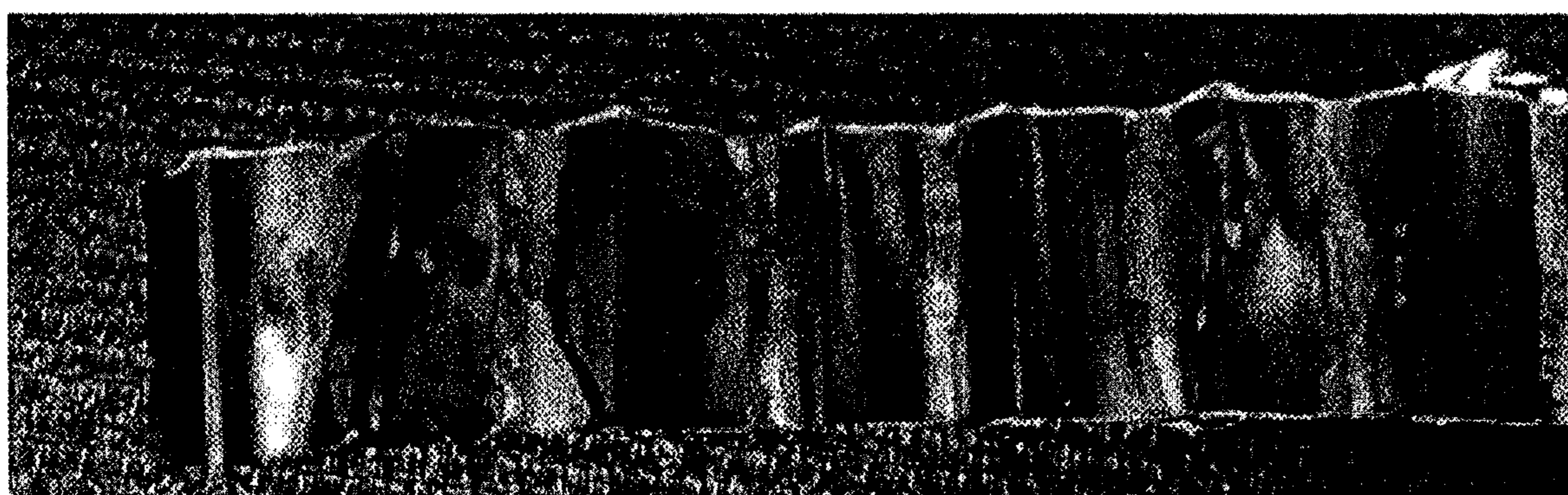
Figure 19. Photograph of CE 1 after Autopsy of Hot Box Tested Battery Showing Separator is Fully Melted to Cathode and Cannot Be Peeled Away From It.
