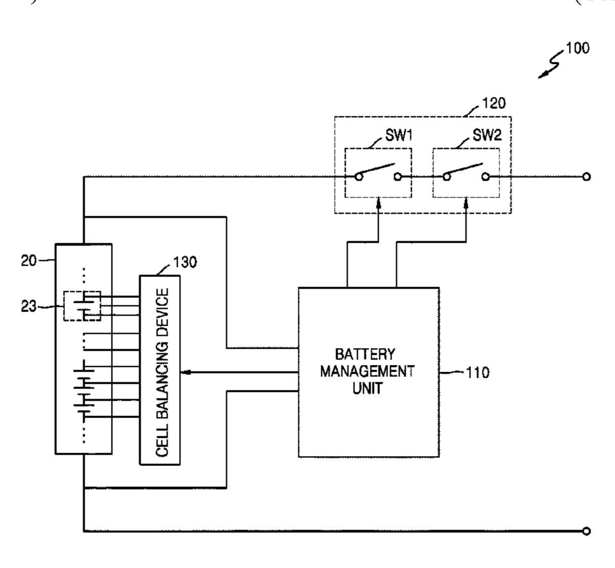
battery management unit is configured to operate the cell balancing device for a preset discharging time to make the battery self-discharge, when the present discharging time passes, the battery management unit is configured to pause the battery from self-discharging for a preset pausing time, and when the preset pausing time passes, the battery management unit is configured to charge the battery.
