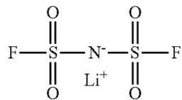
In some embodiments, it is desirable to use a lithium-based salt having the general formula  $(\text{Li}^+)(\text{CF}_3-(\text{CF}_2)_n-\text{SO}_2-\text{N}^--\text{SO}_2-(\text{CF}_2)_n-\text{CF}_3)$ , wherein  $n \geq 0$ . The molecular structure of this general formula is illustrated in Structure 7, below. Structure 8, also below, illustrates the case in which  $n=0$ , which is lithium bis(trifluoromethanesulfonyl)imide (LiTFSI).
