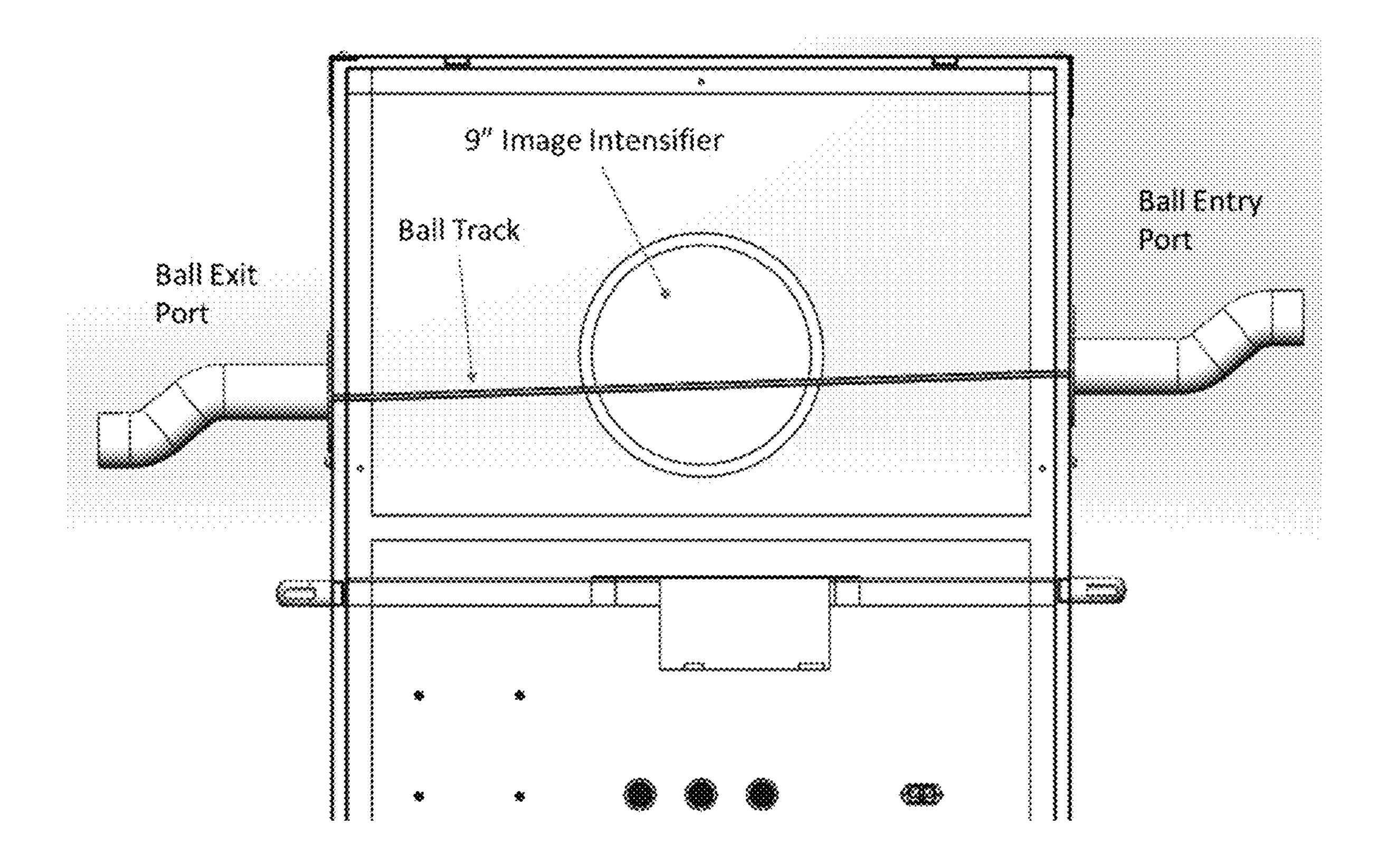
Figure 2: Section View Depicting X-ray Cabinet Configured for Random Ball Rotation
