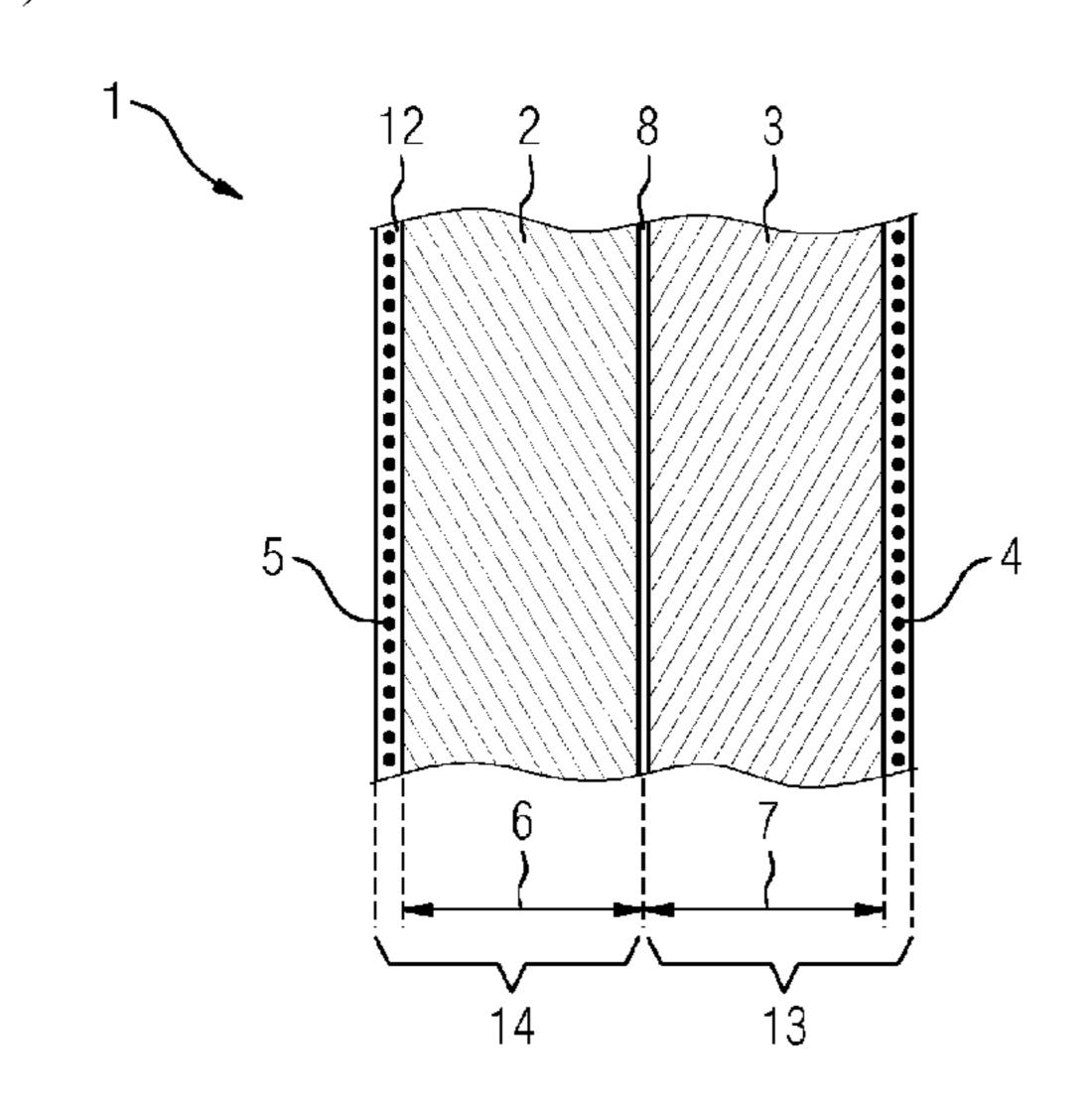
anion-selective membrane directly adjoins the first cationpermeable membrane and the second anion-selective membrane directly adjoins the cathode.
