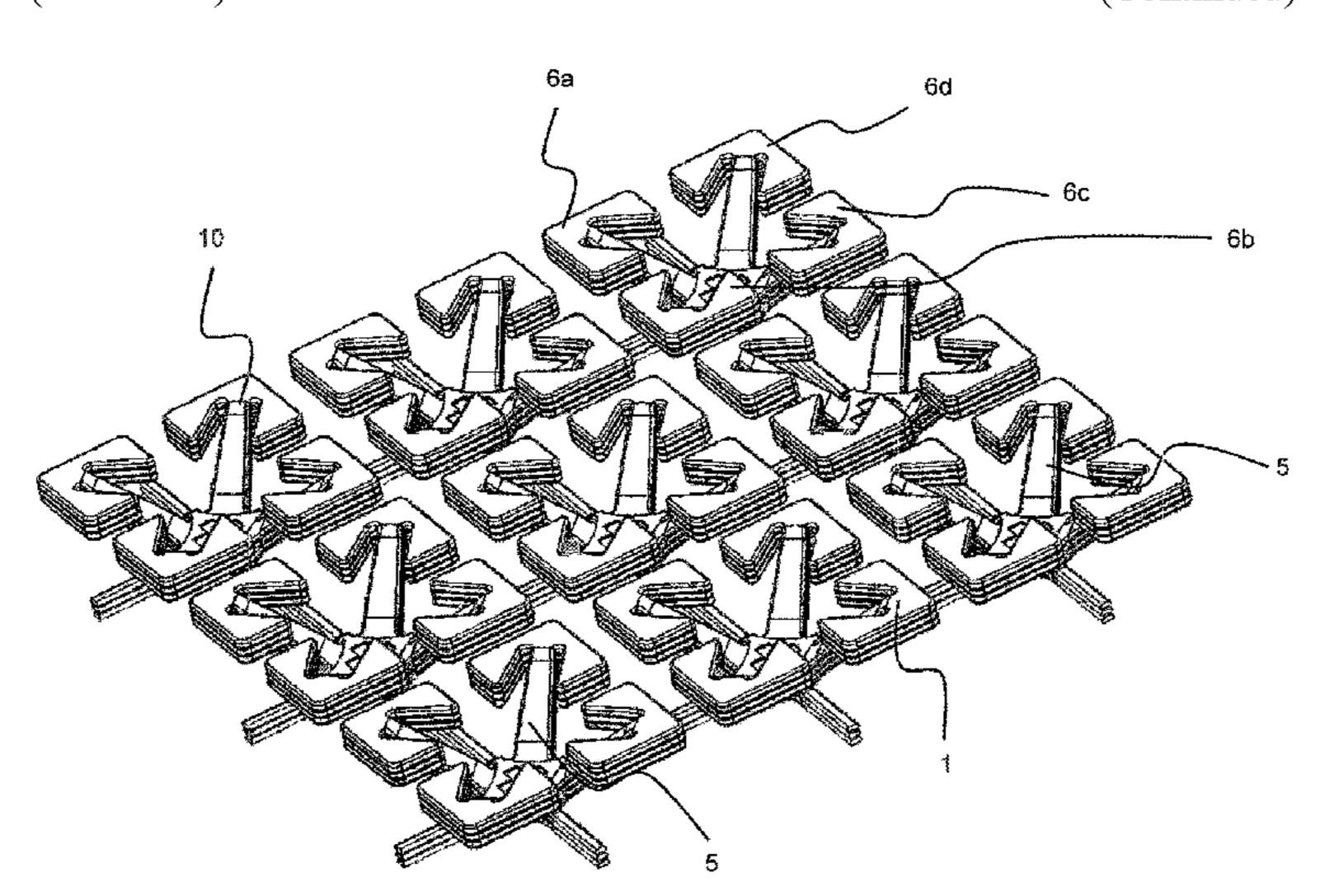
spring elements in such a manner that the spring elements are fixed in their position relative to one another, wherein the connecting elements are formed in one piece and are integrally molded onto the spring elements. The application furthermore includes a stack of spring element arrangements.
