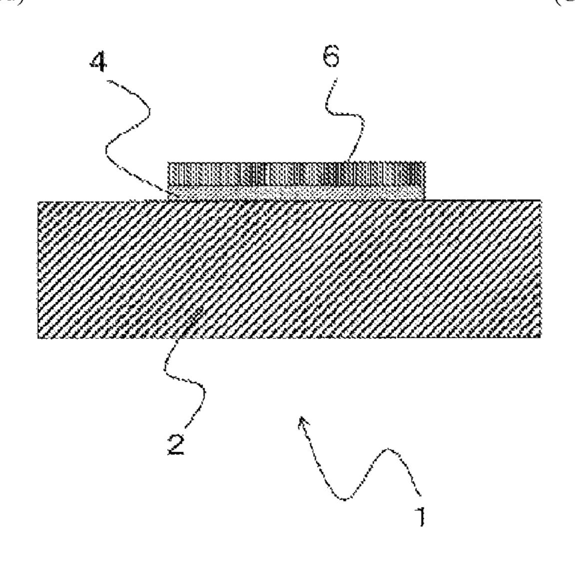
body of silver fine particles; the main component of the resin layer is a polyurethane resin having an elongation at break of 600% or more; and the polyurethane resin has one of the functional groups represented by —COO—H, —COOR, —COO-NH+R<sub>2</sub> and —COO-NH<sub>4</sub>+.
