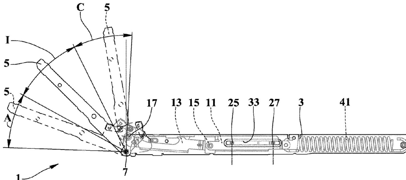
slots (31) of the cradle (11) and into second slots (33) of the first element (3).
