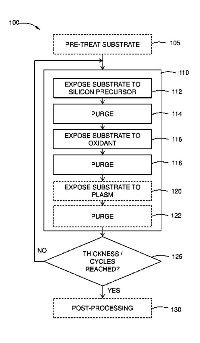
chamber of the silicon precursor; exposing the substrate to an oxidant; and purging the processing chamber of the oxidant.
