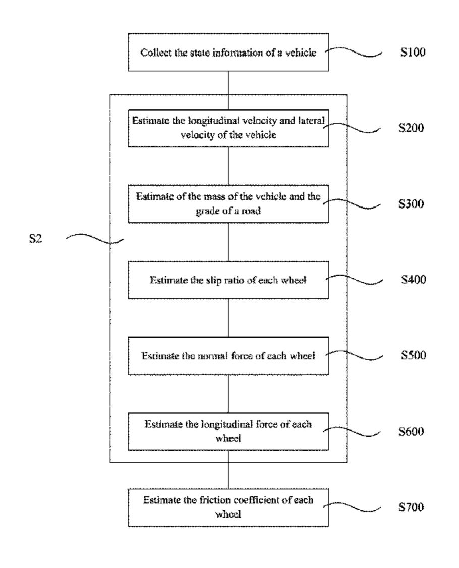
state information, and chassis state information from sensors mounted on the vehicle and specifications set for the vehicle; estimating a longitudinal slip ratio, normal force, and longitudinal force for a tire mounted on each wheel of the vehicle by using the acquired state information of the vehicle; and estimating a road surface friction coefficient for the tire by using the estimated longitudinal slip ratio, normal force, and longitudinal force.
