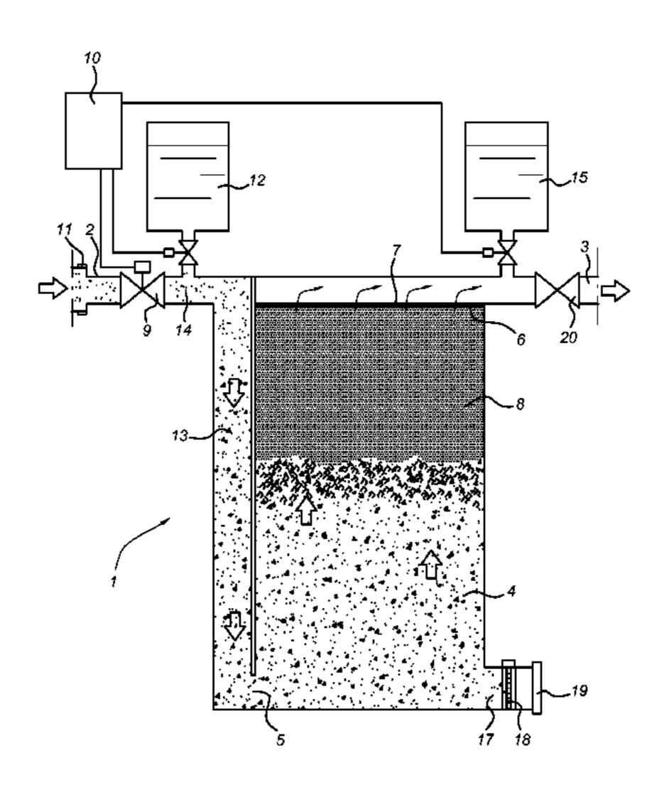
ticulate filter media that partially fills the interior of the filtration chamber; •a flow regulator that regulates the flow rate of aqueous liquid through the filtration chamber and that can operate in a high flow rate mode or a reduced flow rate mode; •a timer that controls the flow regulator; wherein the timer is programmed to alternatingly switch the flow regulator from the high flow rate mode to the reduced flow rate mode.
