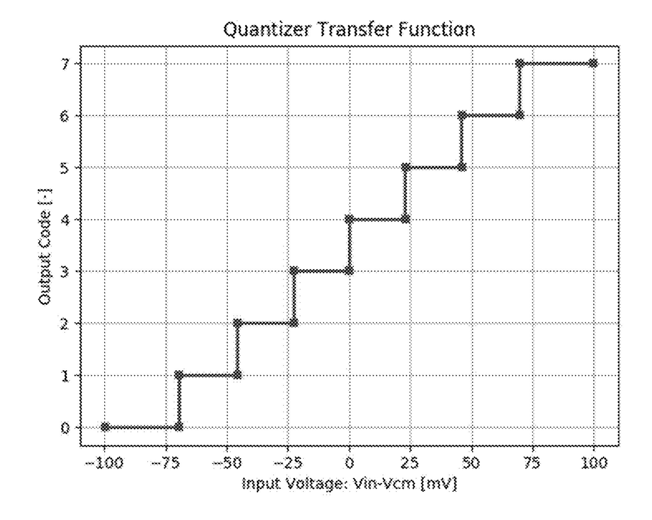
3-bit slit-gate laddered-inverter quantizer with ~23.5 mV quantizer step voltage
