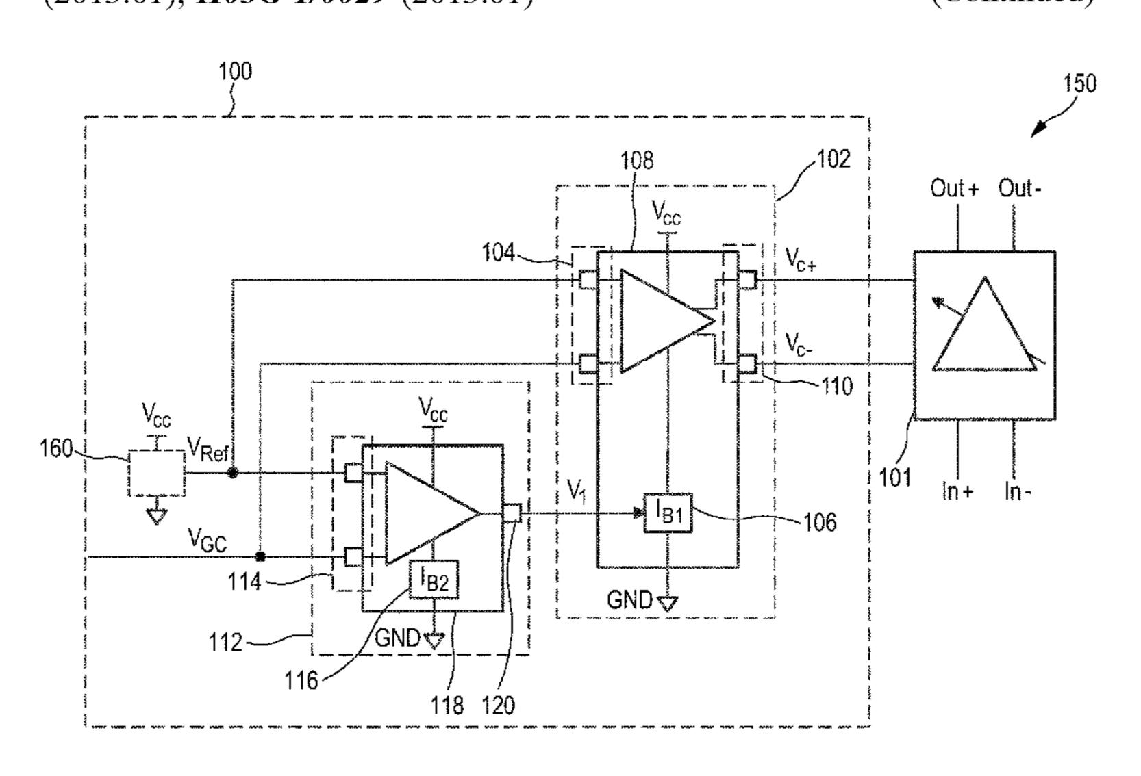
a first biasing current  $(I_{B1})$  that depends on the control voltage signal.
