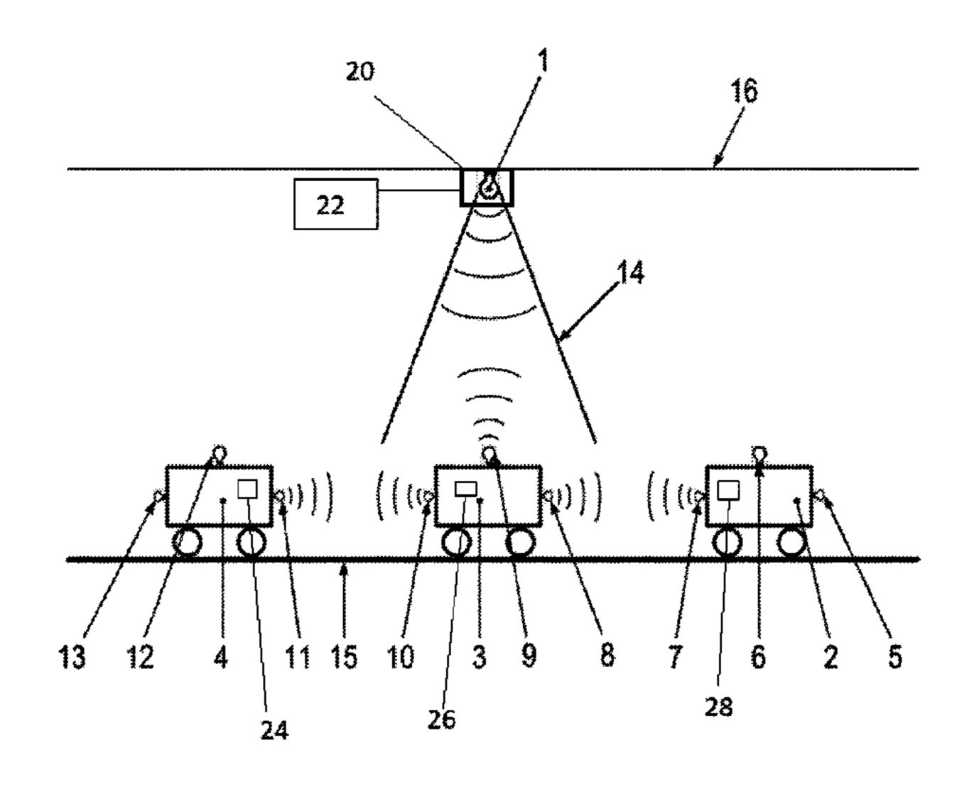
module. A first vehicle that is located within a spatial transmission area of the stationary transceiver module forwards a driving order to a second vehicle that is located outside the spatial transmission area of the stationary transceiver module, and the second vehicle transmits data via the first vehicle and the stationary transceiver module to the central control unit.
