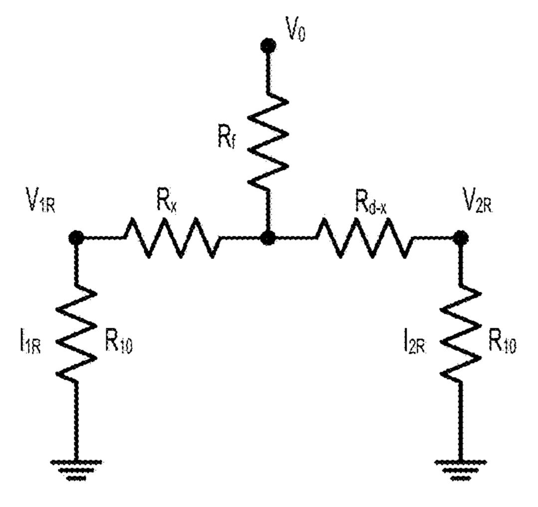
Voltages measured at V<sub>1R</sub> and V<sub>2R</sub> vary with the applied force at position x
