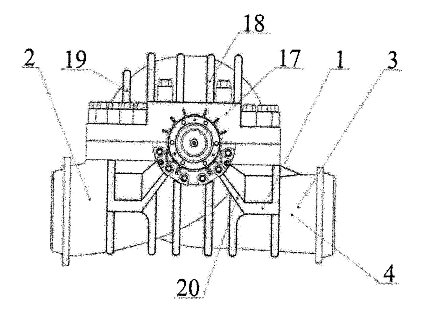
base of the pump housing. The base and the cover of the housing are configured with interior chambers which form an inlet and an outlet. All of the ribs are integral with the cover or the base. The invention is directed toward increasing the reliability and working life of the pump by reducing vibration loads and increasing leak tightness while at the same time minimizing the material requirements of the pump structure.
