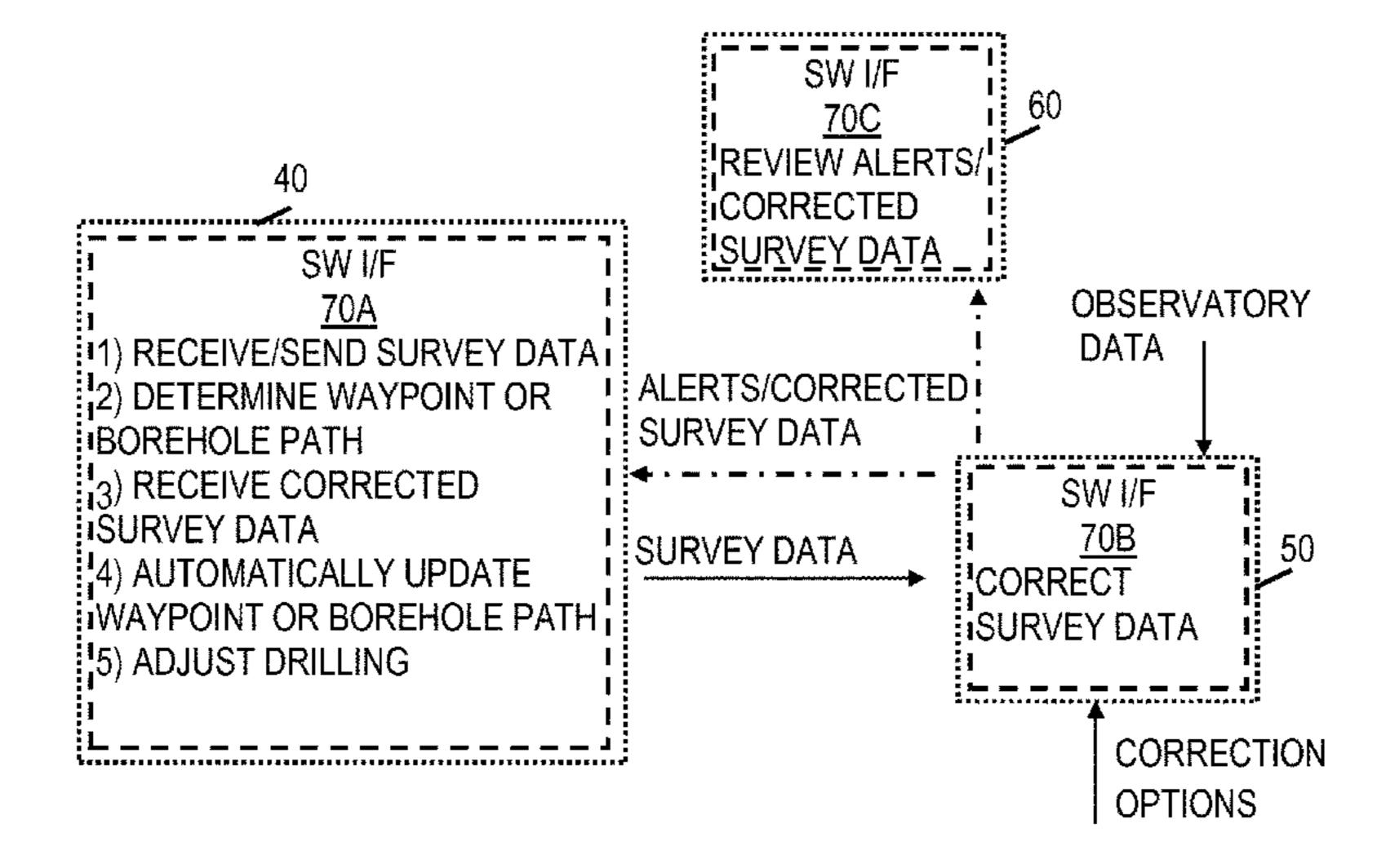
also includes receiving the corrected survey data, and automatically updating the waypoint or borehole path based on the corrected survey data.
