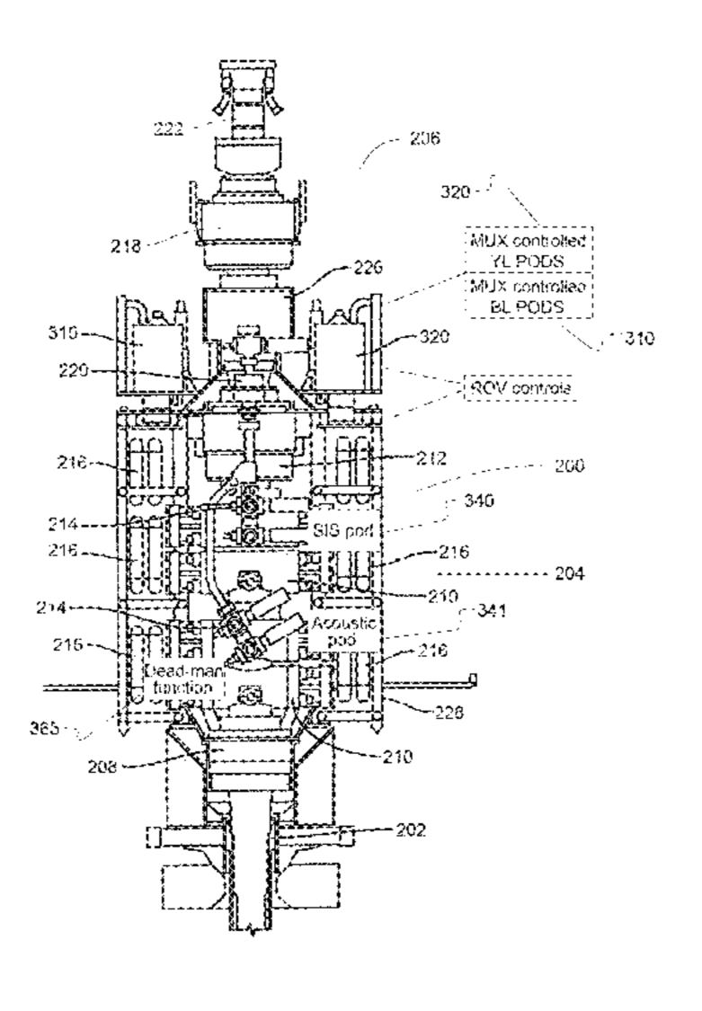
connected, during use, to a surface control system and to be controlled, during use, by the surface control system, wherein the blowout preventer system further includes at least one additional control pod connected to at least one additional surface control system and to be controlled, during use, by the additional surface control system. In this way, an improved blowout preventer system is provided.
