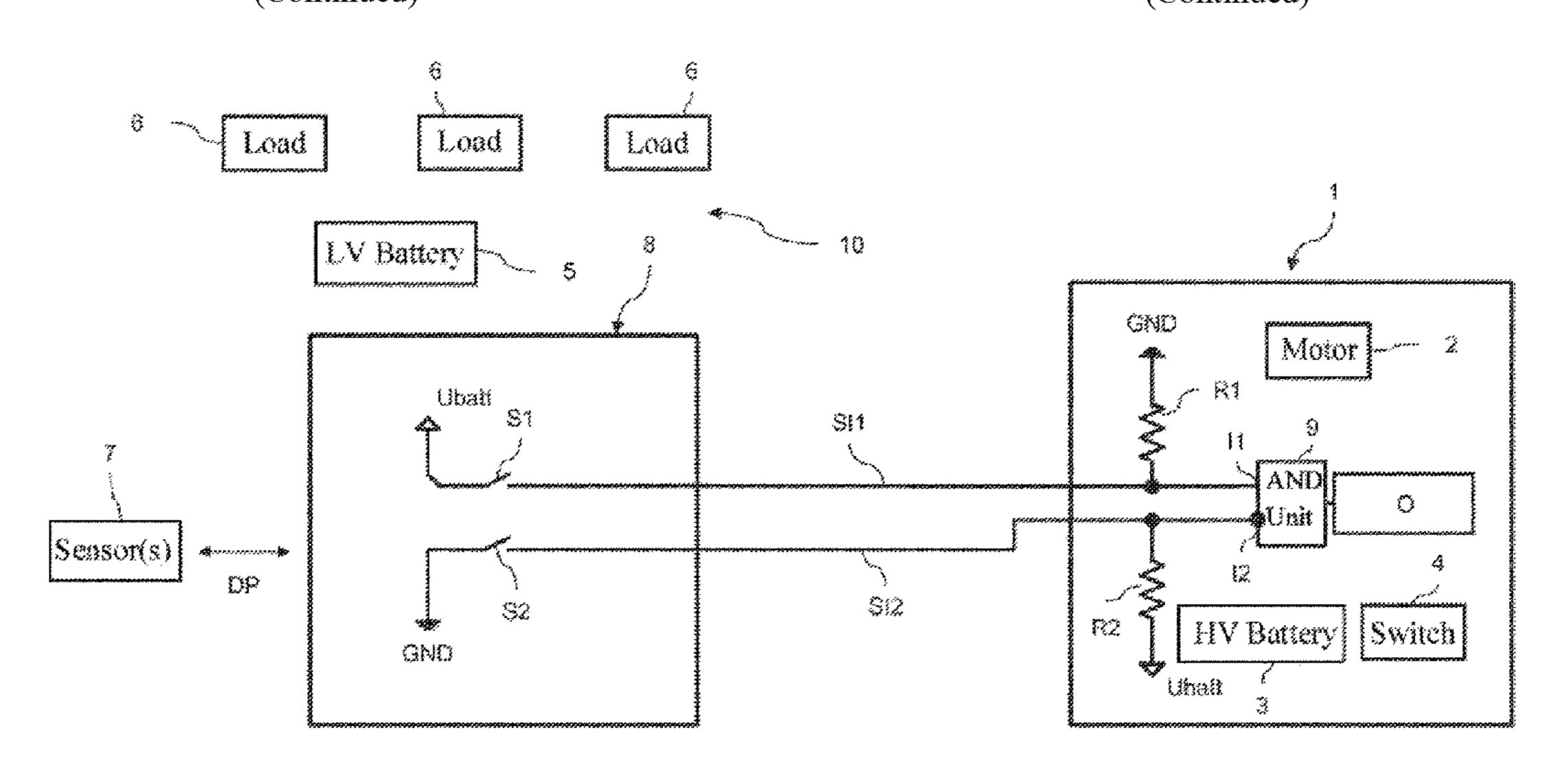
to the predetermined signal change. The signal path includes a first and a second signal line, wherein the predetermined change of the signal on the signal path includes a change of the signal level on each of the first and second signal lines.
