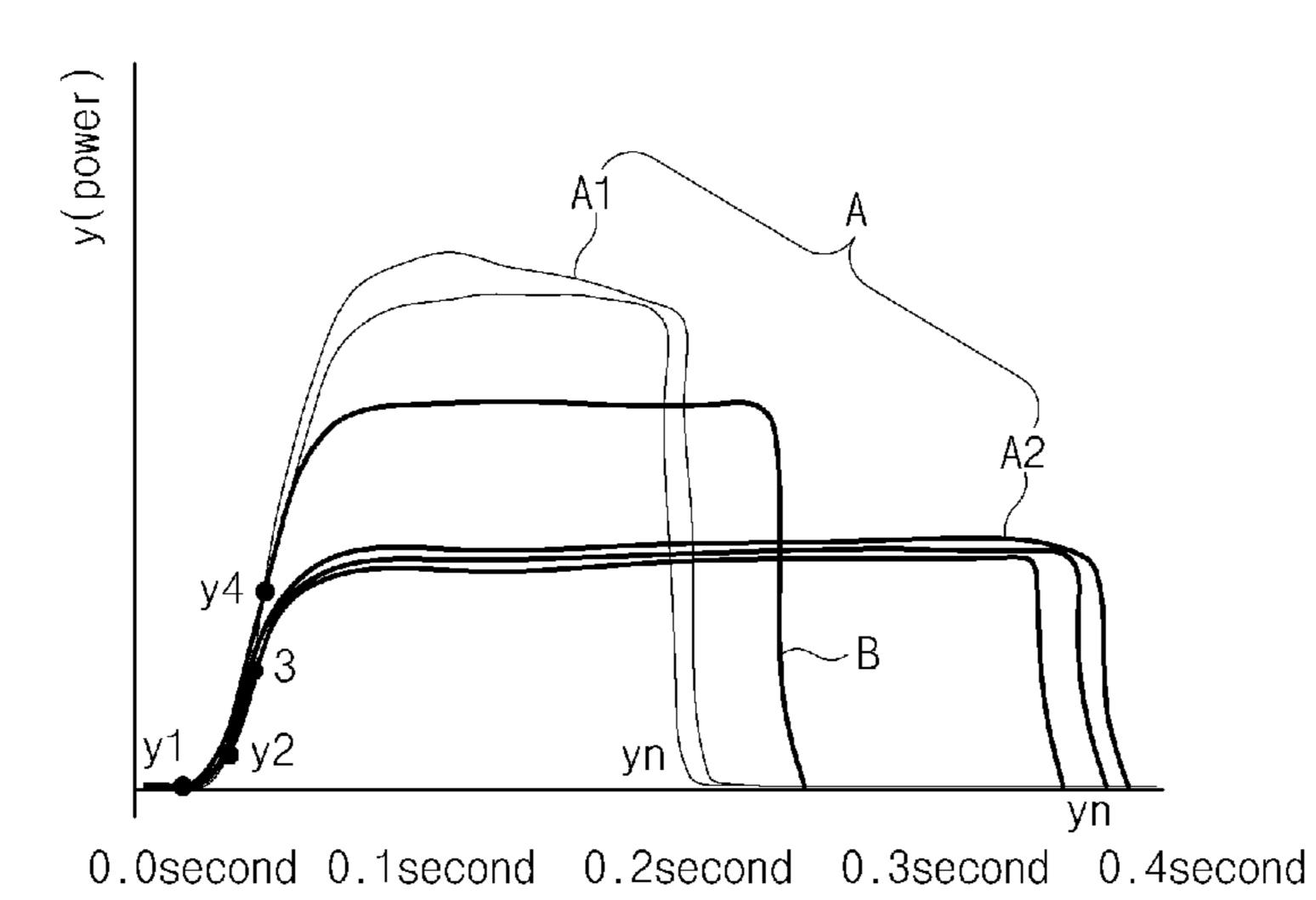
suring unit to display the waveform on a graph; and an inspection unit comparing the measured welding waveform displayed on the graph with a normal welding waveform to inspect whether the defective welding occur in real-time.
