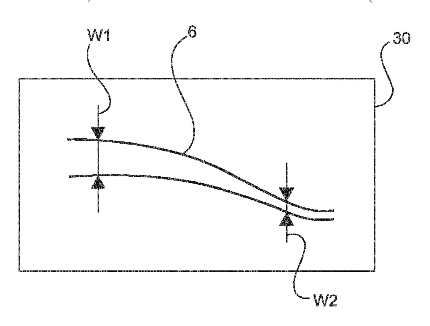
an input interface (40) and a processing unit (50). The input interface is configured to obtain image data (30) representing a two-dimensional representation of a vessel (6). The processing unit (50) is configured to determine a course of the vessel (6) and a width (w1, w2) of the vessel along its course in the image data and is further configured to determine the functional index for stenosis assessment of the vessel based on the width of the vessel in the image data.
