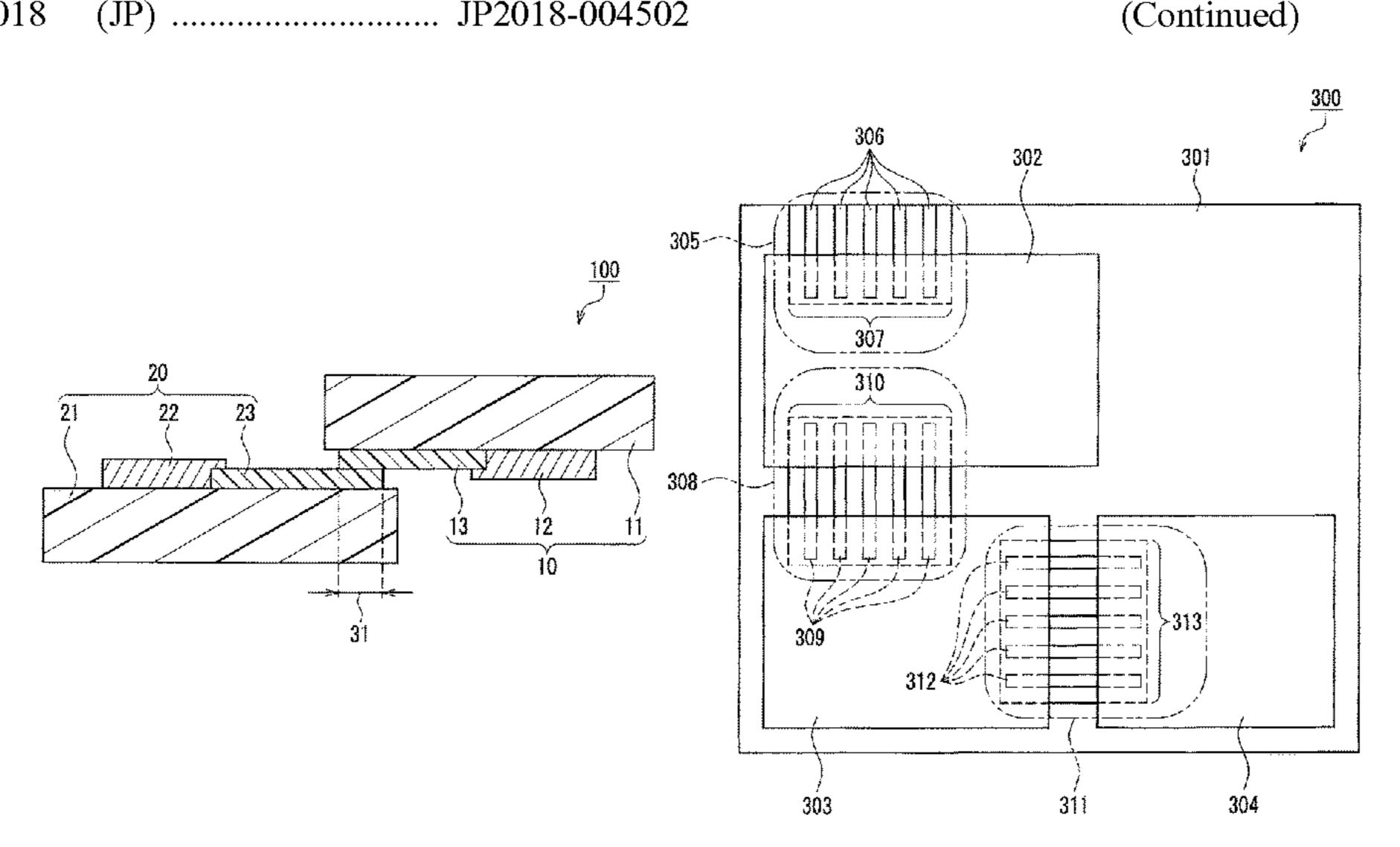
part of the conductive wiring serves as a connection part with another electronic member. Further, an electronic device 100 includes flexible bases 11 and 21, conductive wirings 13 and 23 made of a conductive organic compound formed on the bases, and electronic elements 12 and 22 connected to the conductive wirings, wherein part of the conductive wiring serves as a connection part 30 with another substrate.
