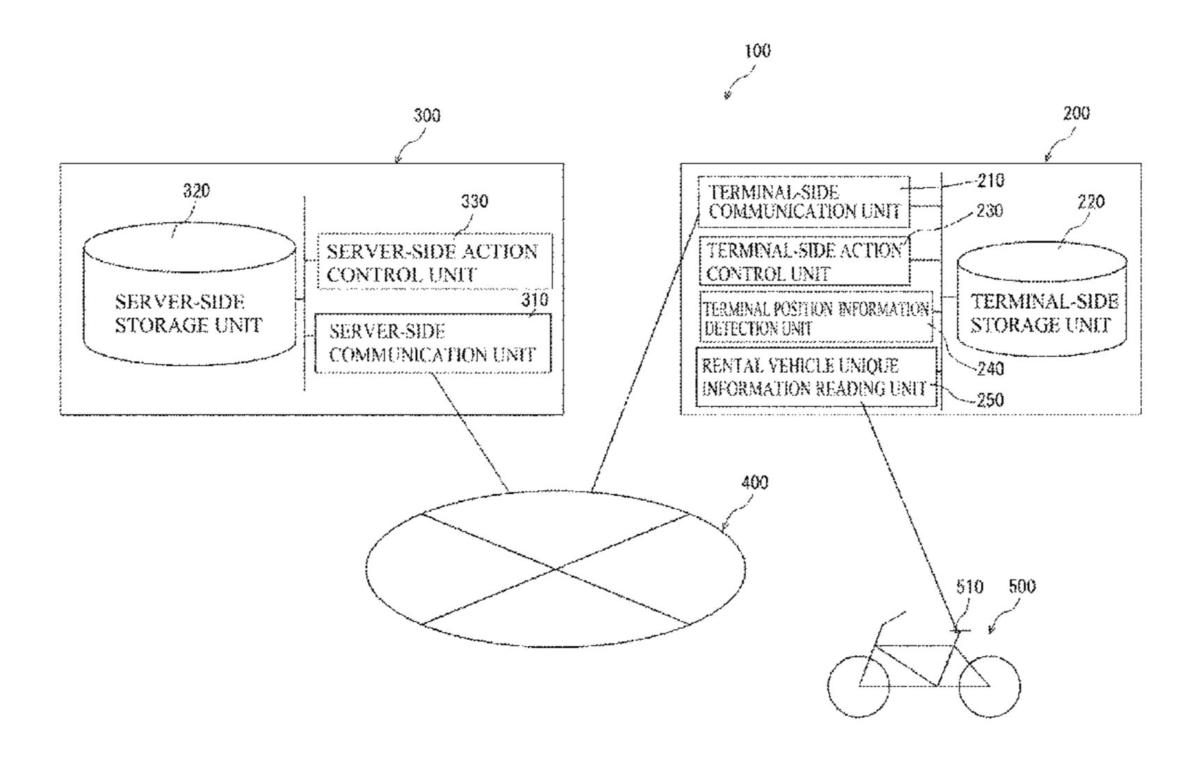
action control unit (330) refers to a user information database (321), a facility unique information database (322), and a rental vehicle unique information database (323) stored in a server-side storage unit (320) based on the received information and imparts points to a return destination facility provider for the rental vehicle (500) and the user.
