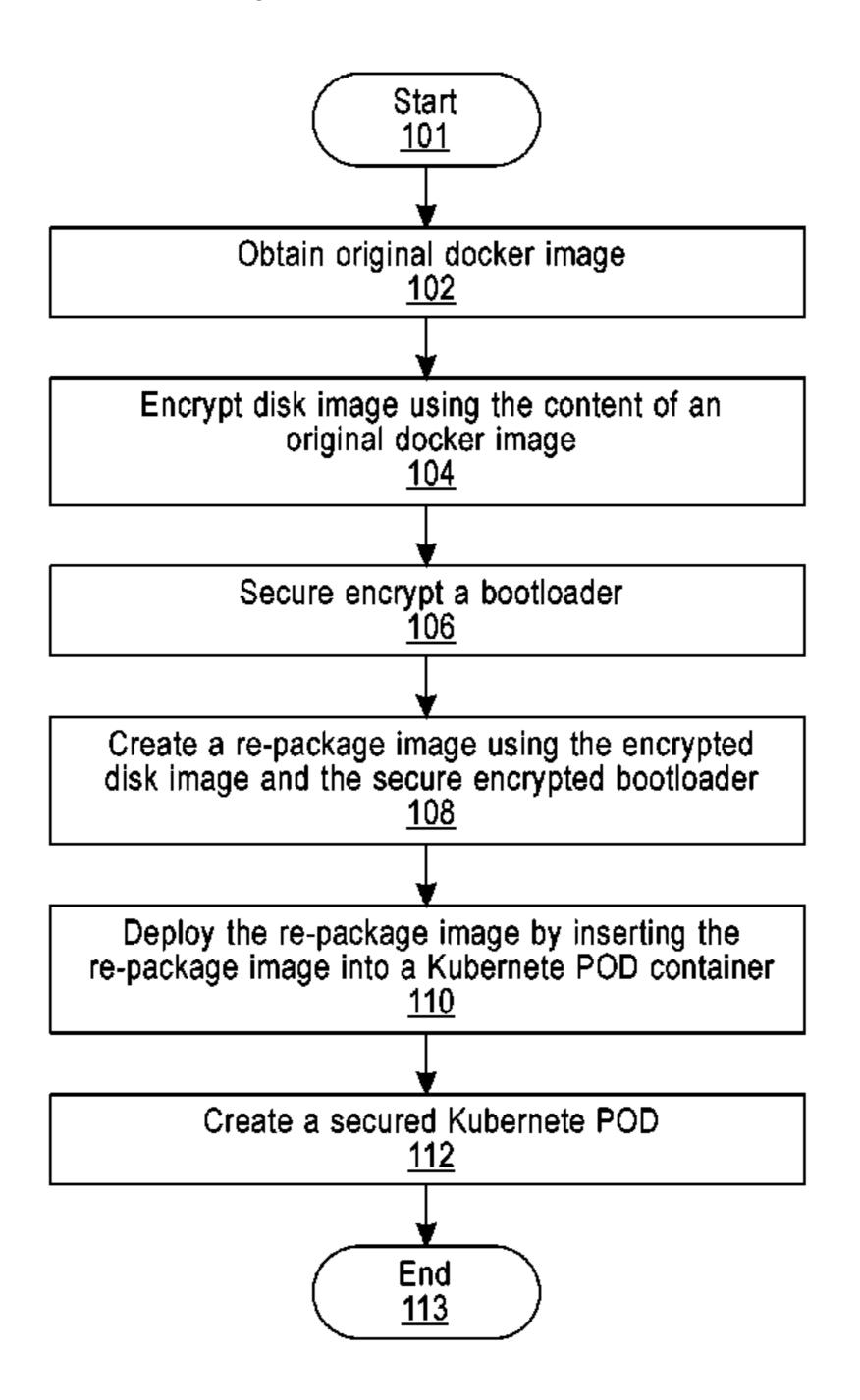
said container and creating a secured Kubernetes pod for protecting workloads, wherein the secured Kubernetes pod has at least one virtual machine containing the pod container.
