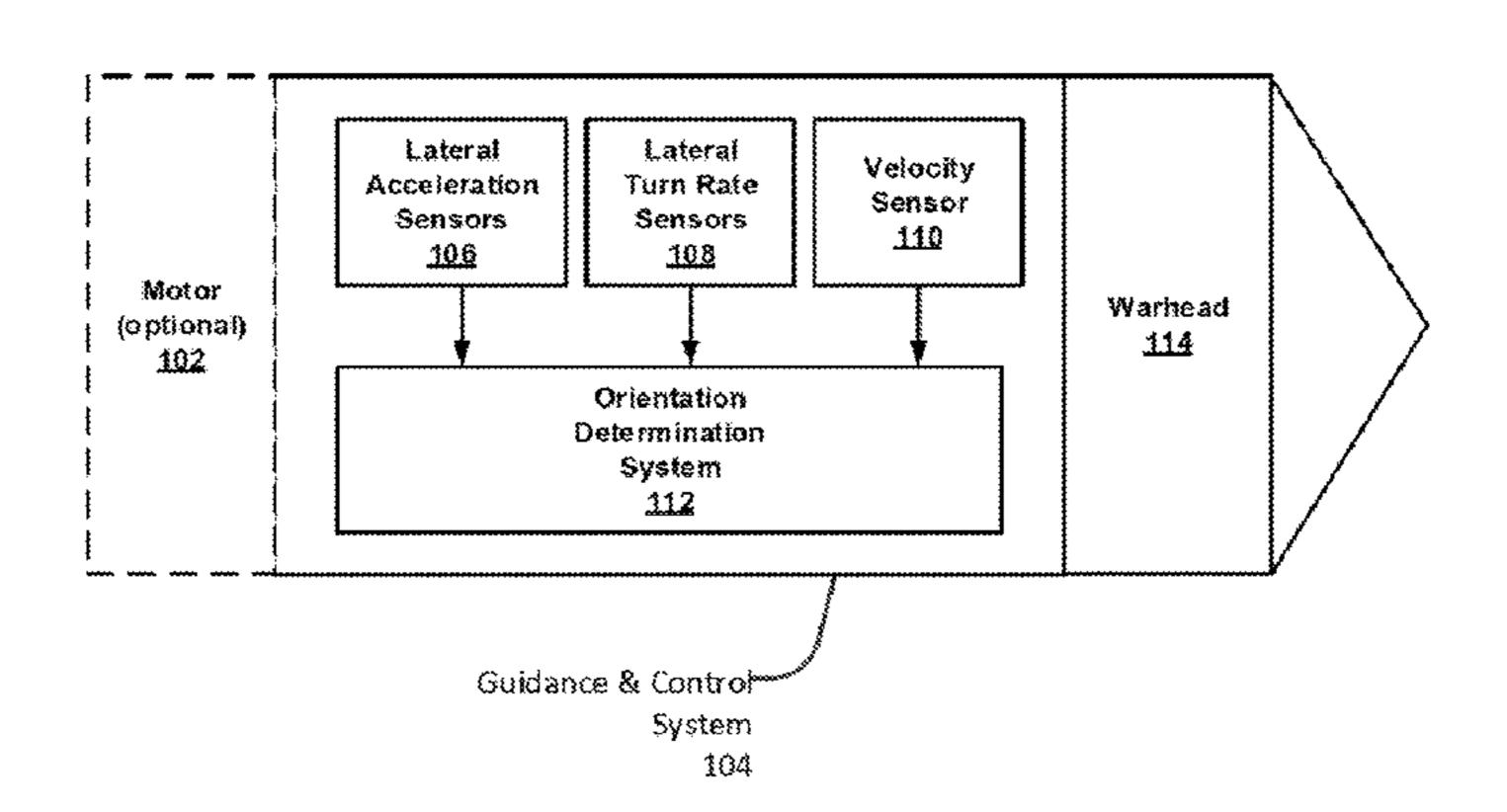
to generate a first type of predicted attitude change. The method further includes obtaining and integrating a lateral turn rate vector measurement of the guided-munition, over the period of time associated with flight of the guided-munition, to generate a second type of predicted attitude change. The method further includes calculating a gravity direction vector based on a difference between the first and second types of predicted attitude change.
