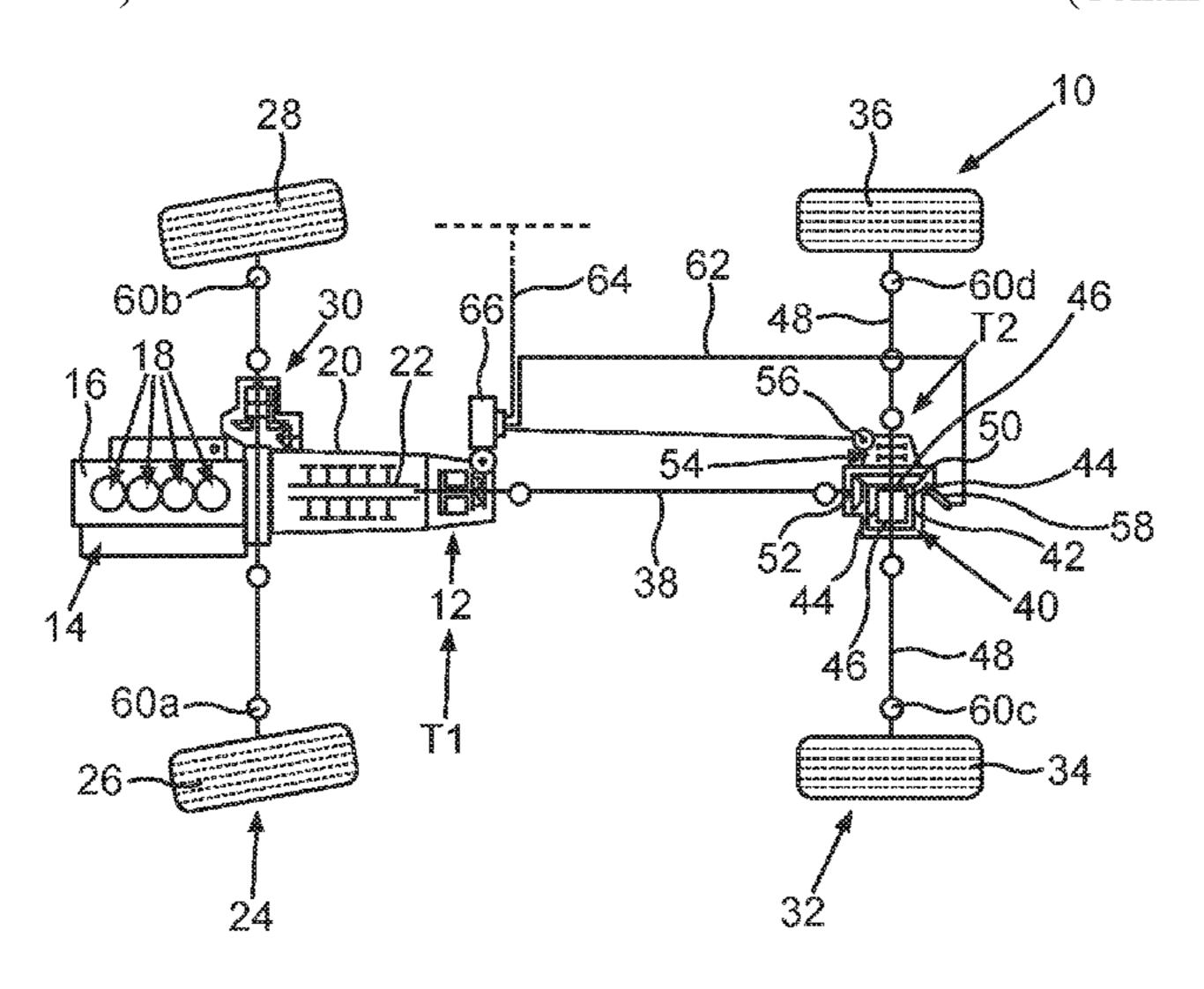
pling torque of the clutch that is lower than the first coupling torque is set: determining at least one coefficient of friction of a roadway the vehicle is located on; and as a factor of the determined coefficient of friction: adjusting a basic torque of the clutch, with the clutch being prestressed in the second position by the basic torque.
