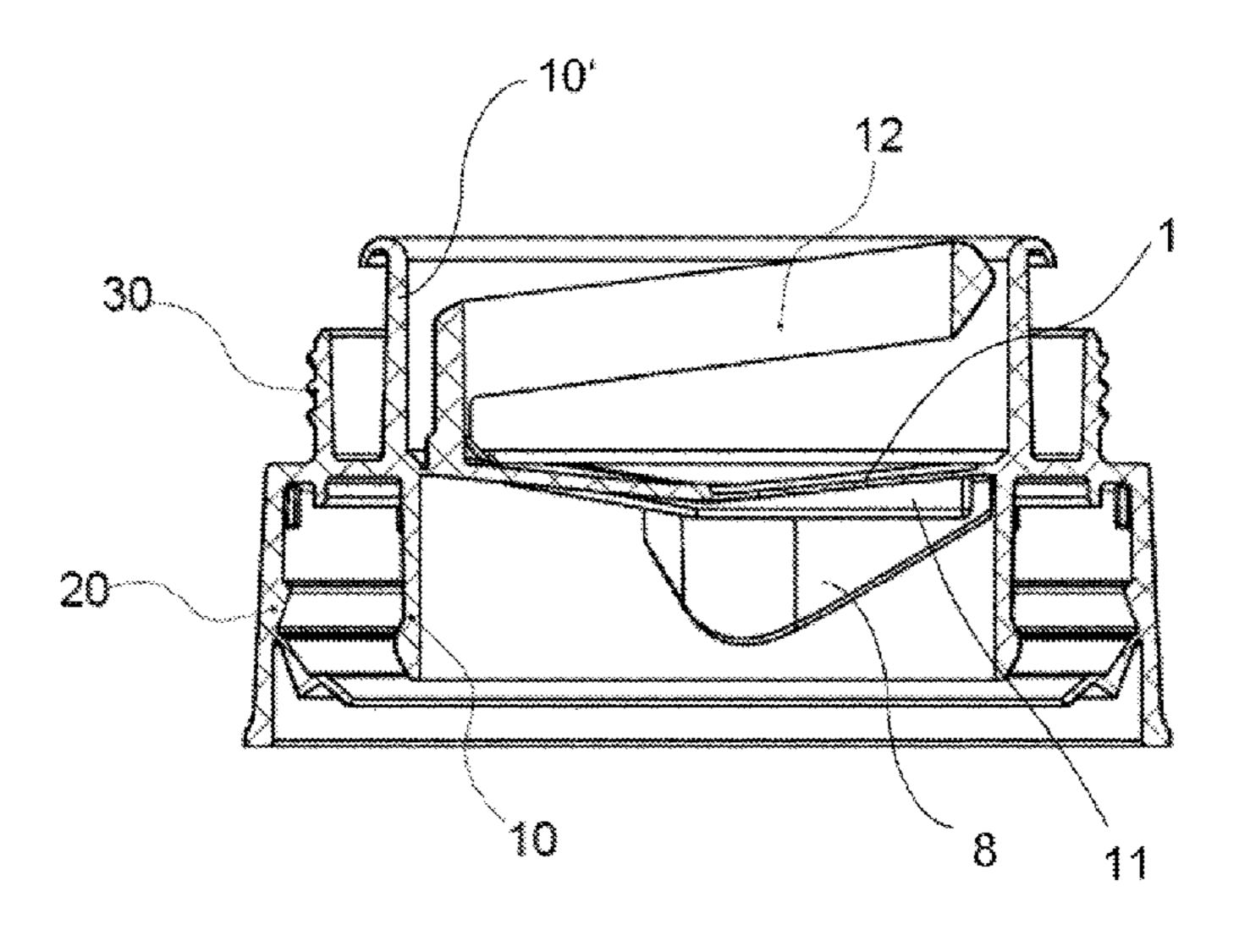
surface at a close distance parallel to the line of weakness and outside the tear-out section run on both sides of the narrow section of the tear-out portion or of the opening and along at least a portion of a transition region between the narrower and the wider sections.
