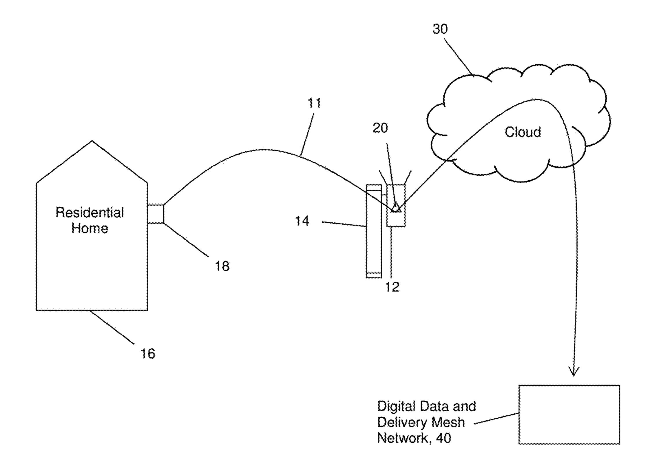
Fig. 4B: Transformer Monitor / Data Collector Device Installation with Residential Locations.
