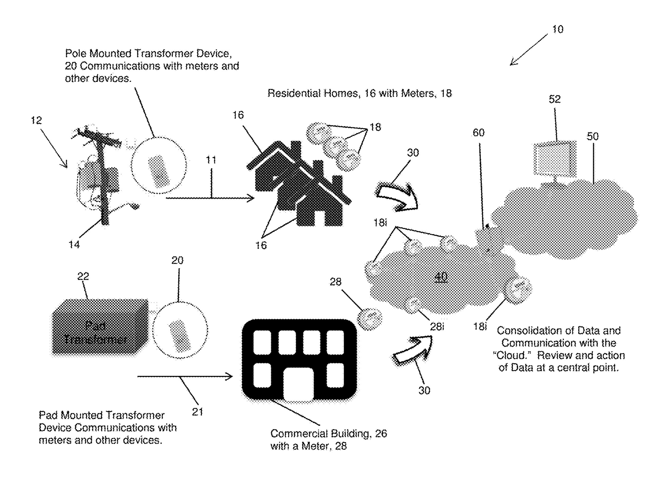
Figure 1A: Example of Network having Residential and Commercial Structures with Transformer Monitor / Data Collector Device
