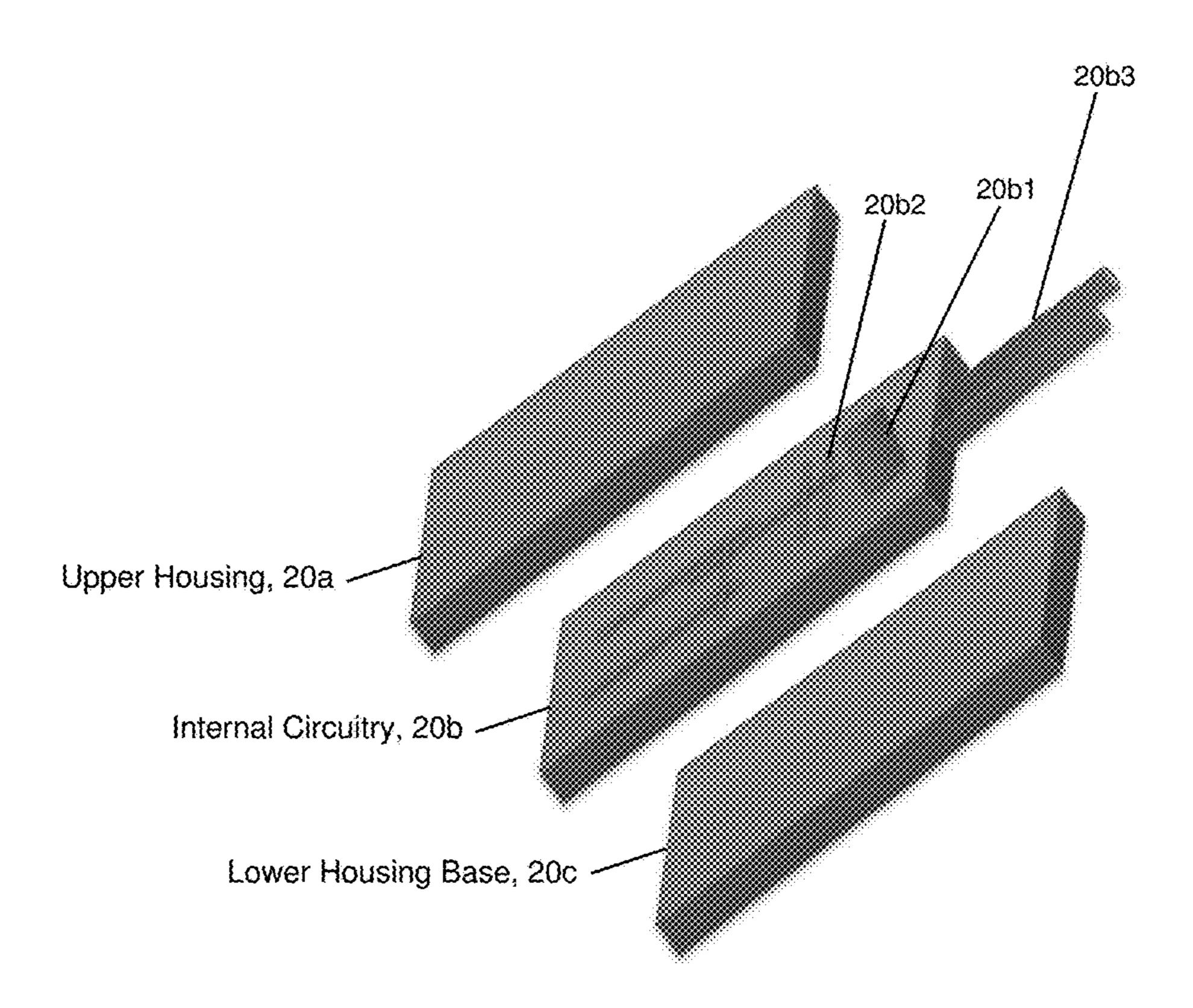
Figure 2: Transformer Monitor / Data Collector Device
