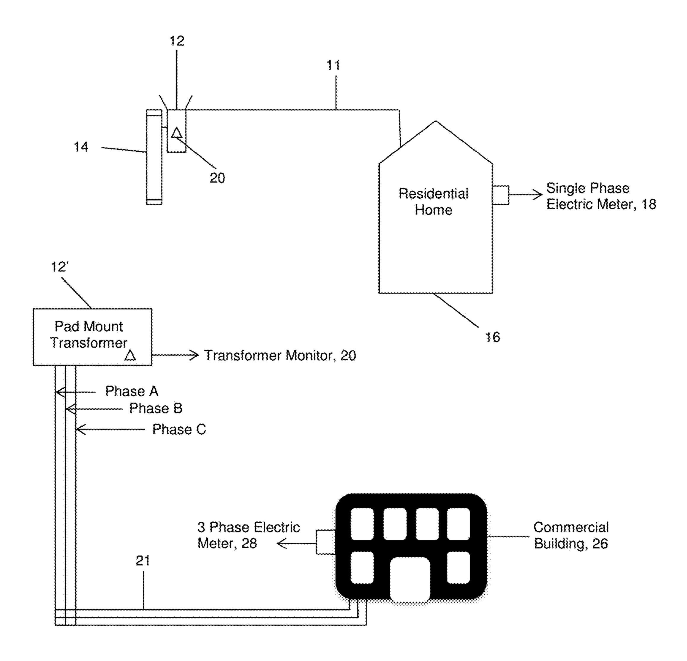
Fig 4A: Transformer Monitor / Data Collector Device Interaction with Residential and Commercial Locations.
