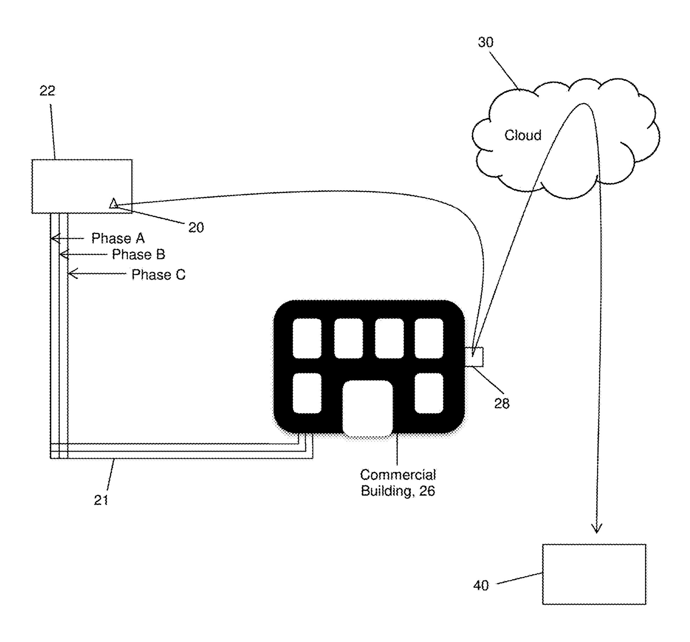
Fig. 4C: Transformer Monitor / Data Collector Device Installation with Commercial Locations.
