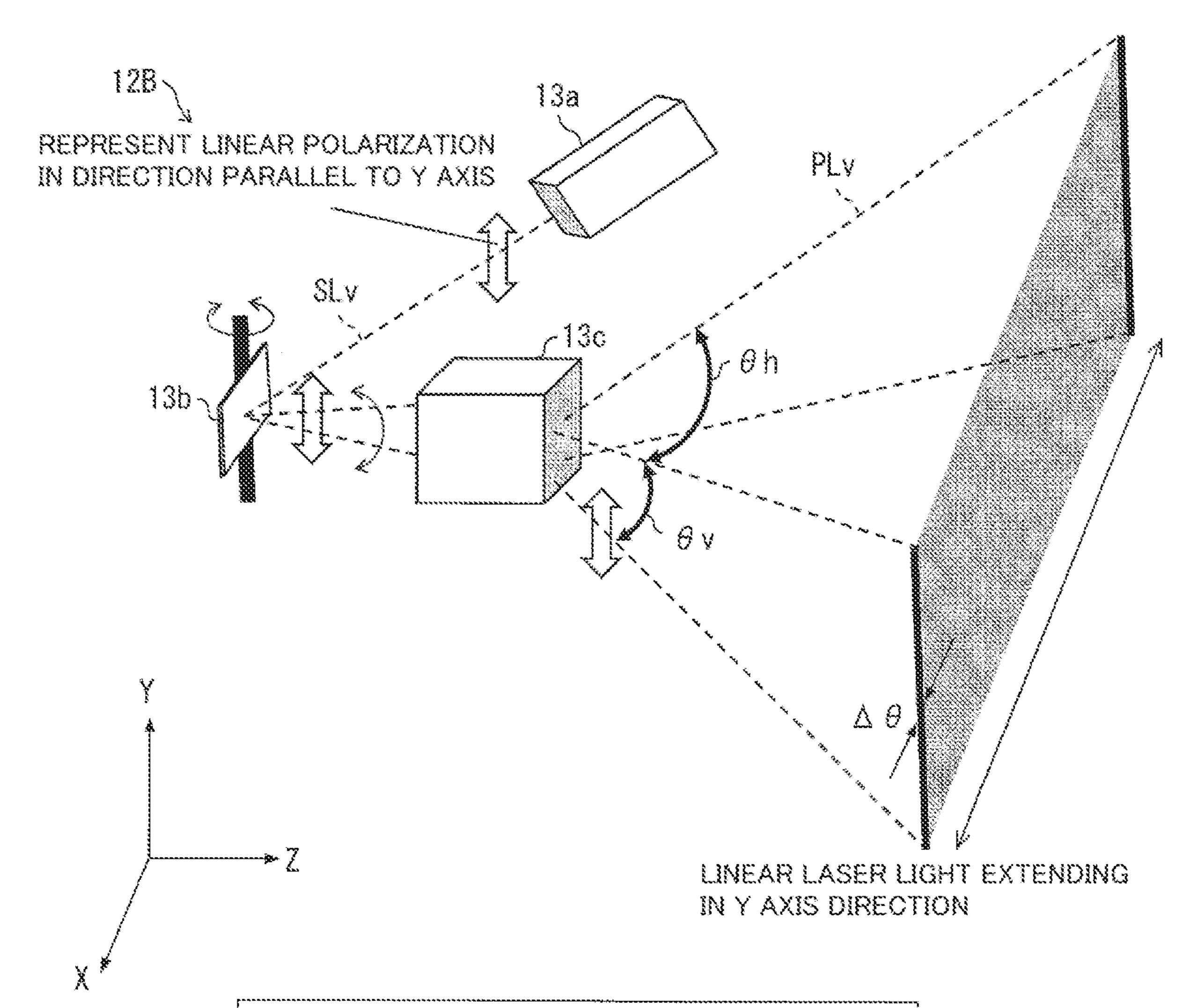
128: FAN-SHAPED PULSE LIGHT RADIATION UNIT
