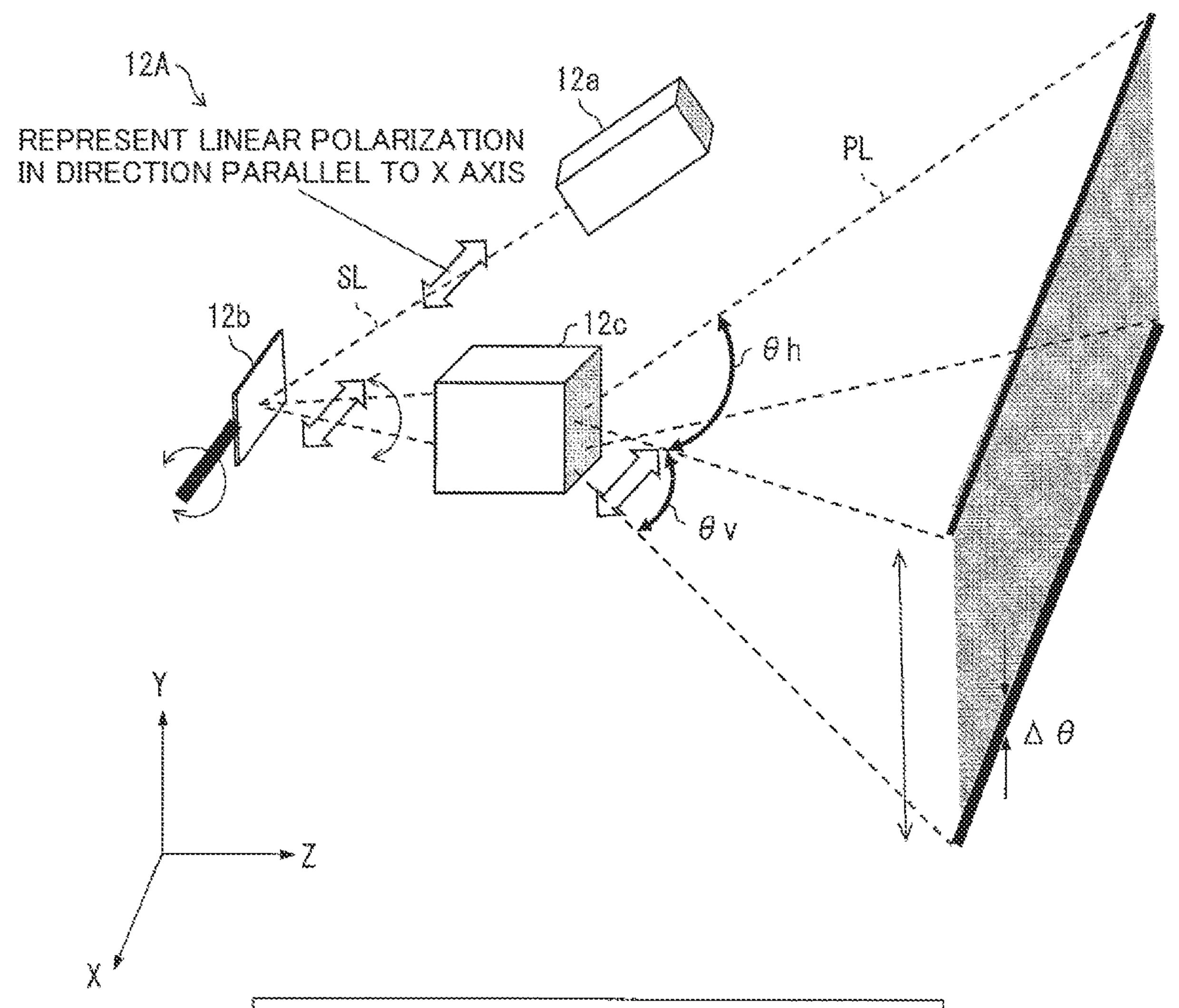
12A: FAN-SHAPED PULSE LIGHT RADIATION UNIT
