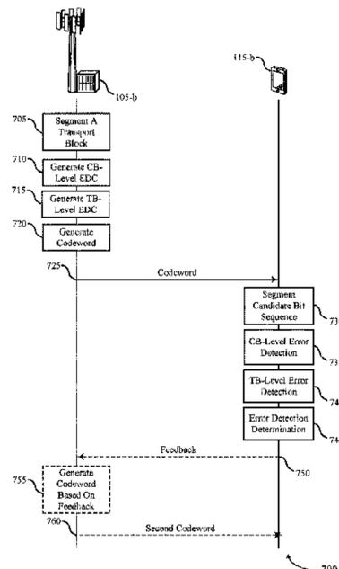
(CB-level) error detection code (EDC) for a subset of the data segments. The encoder may generate a transport block-level (TB-level) EDC for the TB using the data segments. Each of the code blocks (CBs) may be of the same size and may include one of the data segments. A subset of the CBs may include a data segment from the subset of the data segments and one of the CB-level EDCs. The remaining CBs that are not part of the subset may include a remaining data segments and the TB-level EDC.
