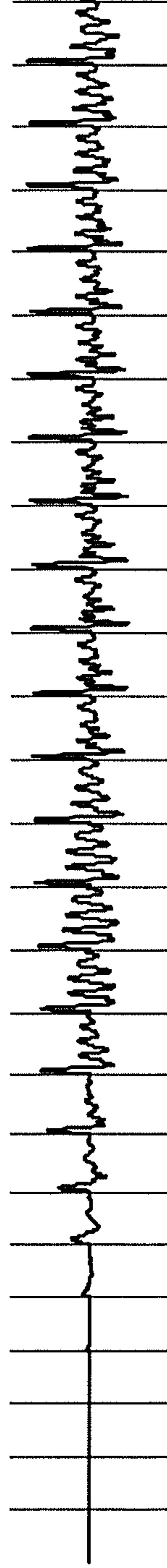
SYNTHESIZED SPEECH WAVEFORM (MINIMUM PHASE) BASED ON PULSE EXCITATION VOCODER
