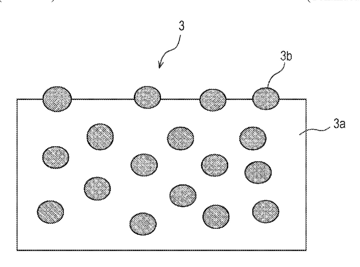
trusions on an outer surface of the member, the outer surface of the electro-conductive member is constituted by the matrix and the domains exposed to the outer surface of the electrophotographic electro-conductive member, the electrophotographic electro-conductive member has an impedance of  $1.0\times10^3\Omega$  or more and  $1.0\times10^8\Omega$  or less, and some of the domains satisfy two specific requirements.
