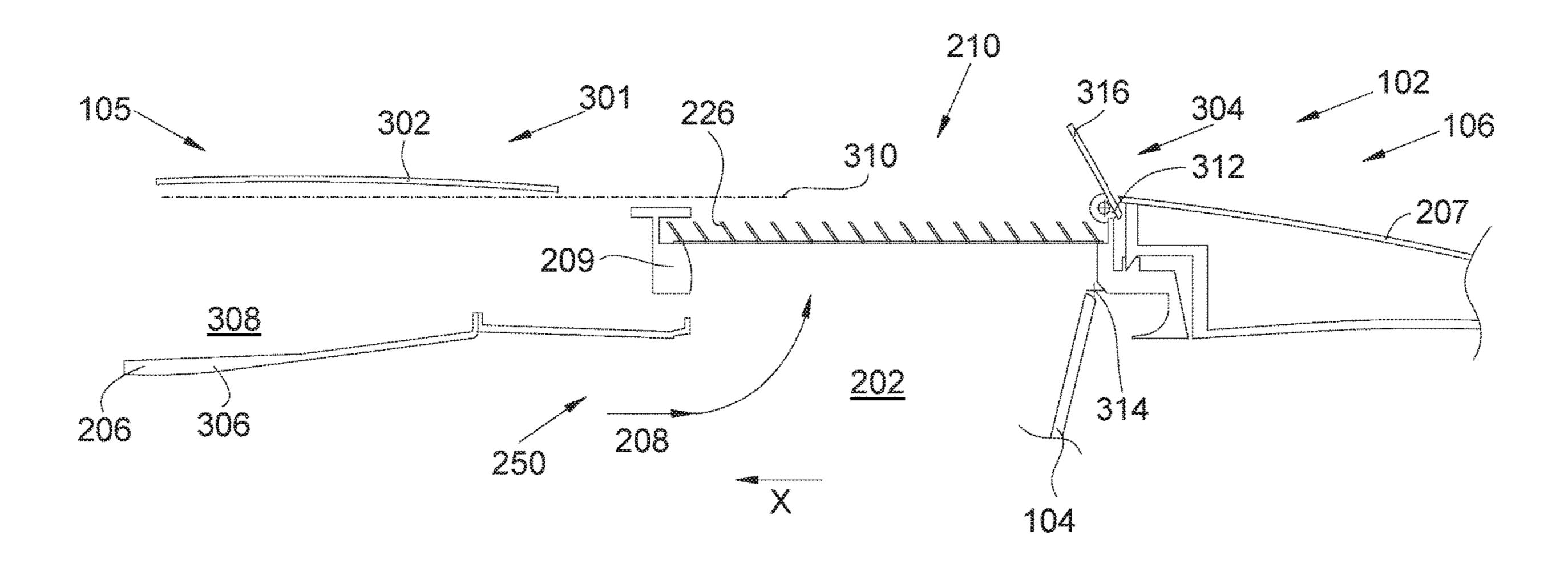
the fan cowl and improve orientation of flow of air passing through the window by orienting the outer flaps.
