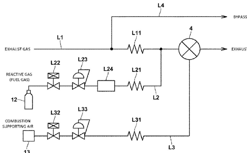
exhaust gas detector associated with a variation in the supply amount of the reactive gas.
